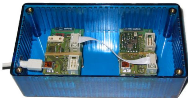
Figure 19: DNS node demonstrator [HW05]. The DSN node is situated on the left side, the target node with a mounted sensor board on the right side.
