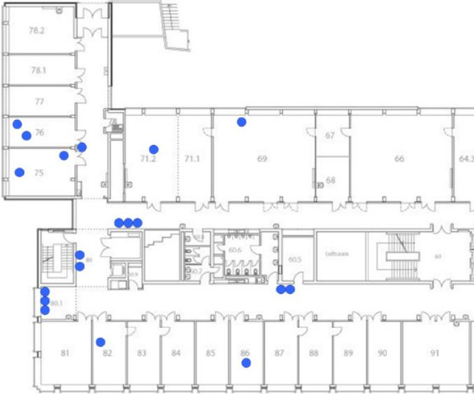
Figure 20: Placement of the 19 BTnodes that form the ETHZ testbed [HW05]. The network is deployed throughout the G floor of the ETZ building at ETH zurich.
