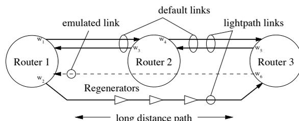
**Fig 3.1** A unidirectional link with a tunnel
