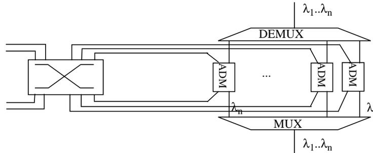
FIGURE 4. Station design using SONET/SDH rings
