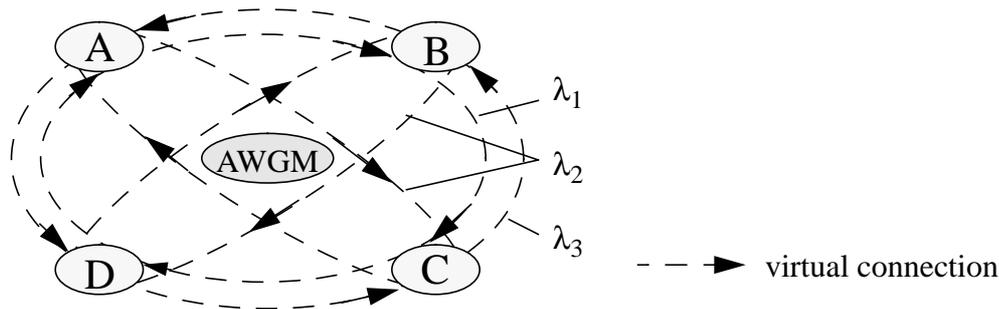
FIGURE 3. Basic topology of a network made up by a 4x4 AWGM. For better visibility only virtual connections are shown.
