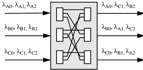
FIGURE 1. The logical structure of a 3x3 Arrayed Waveguide Grating Multiplexer
