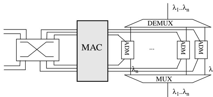
FIGURE 5. Station design using a parallel MAC machine
