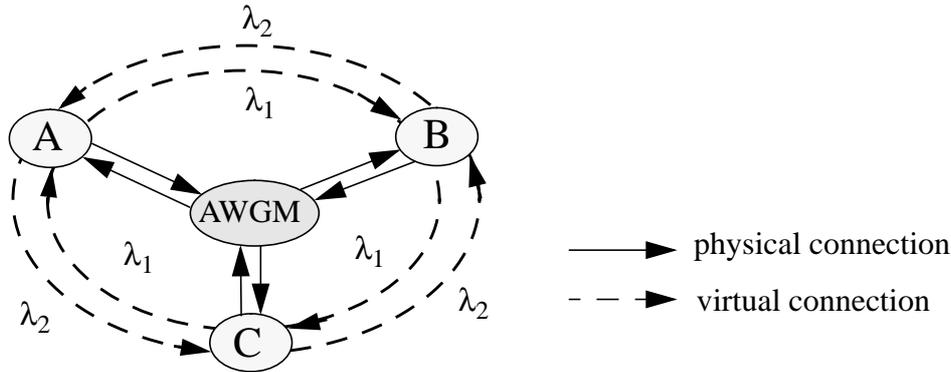
FIGURE 2. Basic topology of a network made up by a 3x3 AWGM
