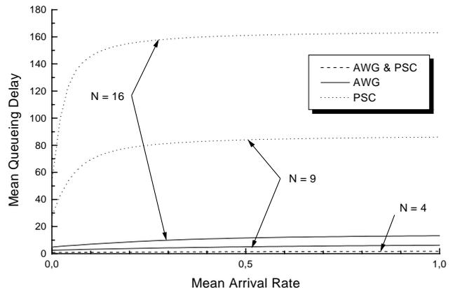
Fig. 10. Mean queueing delay (packet transmission time) vs. average arrival rate (packet/packet transmission time)
