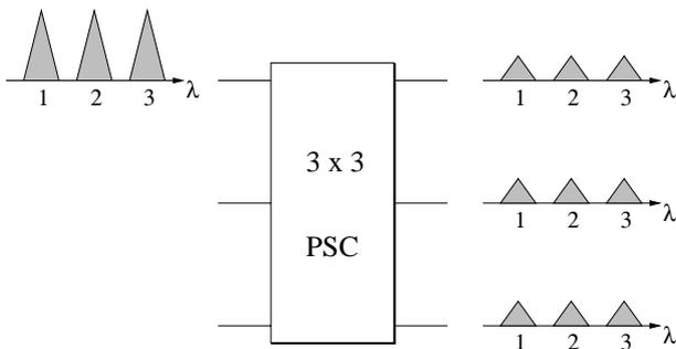
Fig. 1. Broadcasting and splitting loss of a  $3 \times 3$  passive star coupler (PSC)
