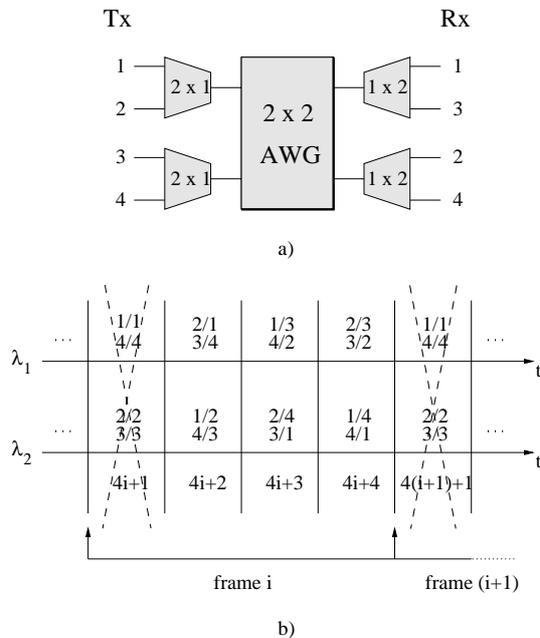
Fig. 7. a) AWG based architecture with cyclic receiver attachment, b) fixed channel assignment with reduced frame length ( $N=4$ )
