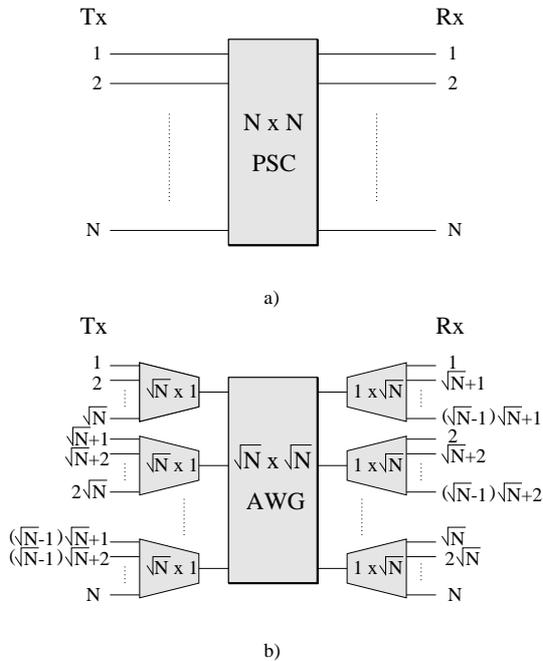
Fig. 5. Single-hop network architecture: a) PSC based, b) AWG based
