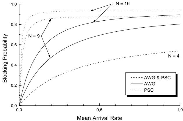
Fig. 12. Blocking probability vs. mean arrival rate (packet/packet transmission time)
