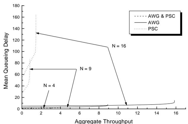
Fig. 11. Mean queueing delay (packet transmission time) vs. aggregate throughput (packets/packet transmission time)
