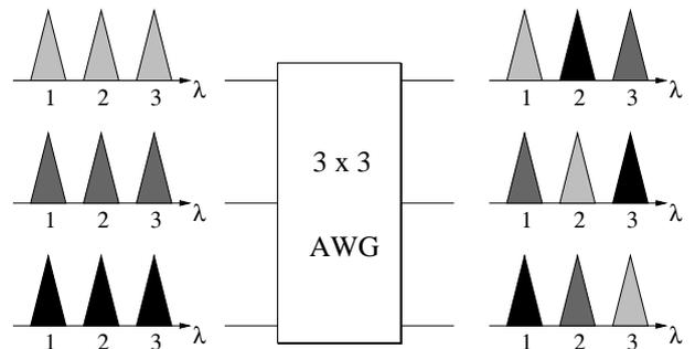
Fig. 2. Wavelength routing and spatial wavelength reuse of a  $3 \times 3$  arrayed-waveguide grating (AWG)
