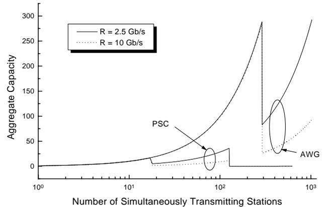
Fig. 8. Aggregate capacity (packets/packet transmission time) vs. number of simultaneously transmitting stations ( $R$  denotes the transmission rate)
