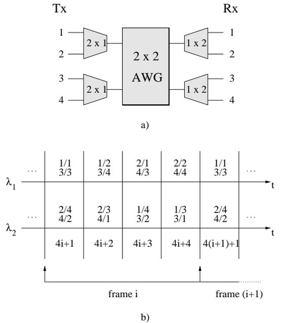
Fig. 6. a) AWG based architecture without cyclic receiver attachment, b) fixed channel assignment ( $N=4$ )
