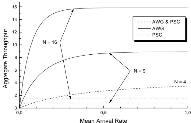
Fig. 9. Aggregate throughput (packets/packet transmission time) vs. average arrival rate (packet/packet transmission time)
