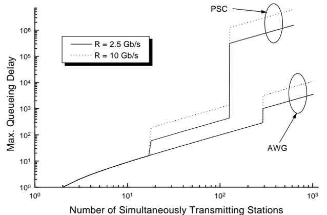
Fig. 14. Maximum queueing delay (packet transmission time) vs. number of simultaneously transmitting stations ( $R$  denotes the transmission rate)
