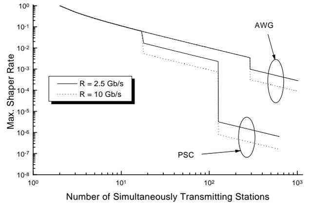
Fig. 13. Maximum shaper transmission rate (packet/packet transmission time) vs. number of simultaneously transmitting stations ( $R$  denotes the transmission rate)
