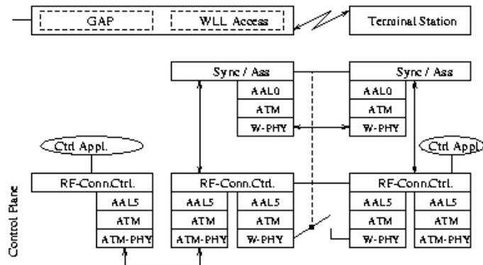
Figure 8. Extended Control Plane for WLL
