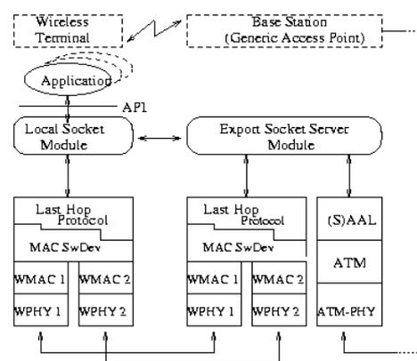
**Figure 5: Remote Socket Architecture (ReSoA)**
