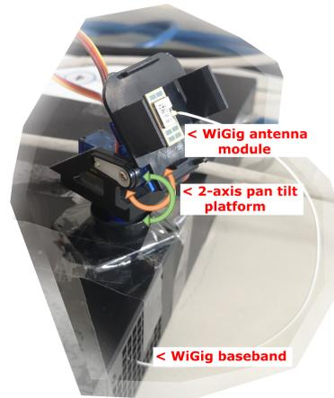
Fig. 2: hWiGig's key component is the 2-axis mechanical rotation of the WiGig antenna module.
