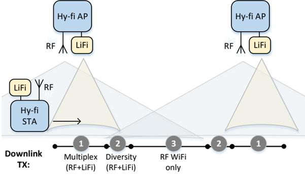
Figure 3.  $\text{Hy-Fi}$  in a mobile scenario with different modes selected for different STA positions.
