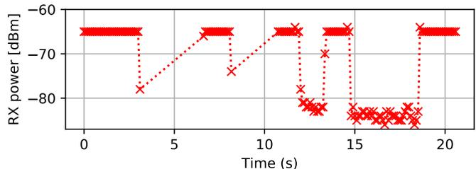
Figure 20. LiFi SISO link with temporary signal blockage.
