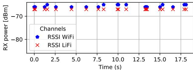
Figure 22.  $H_{y-Fi}$  under continuous jamming on the RF channel with disabled interference management (baseline).
