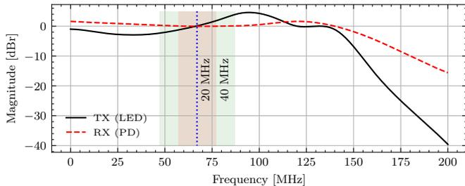
Figure 12. The frequency response of the LiFi front-end (TX & RX).
