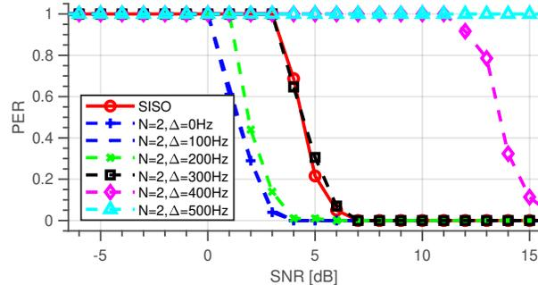
Figure 13. Impact of CFO on a SIMO 802.11 transmission when two same signals with different CFO are received at receiver (MCS=0).
