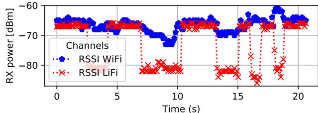
Figure 21.  $\text{Hy-Fi}$  link with temporary signal blockage.
