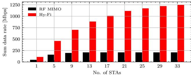
Figure 15. Comparing system-level performance of  $2 \times 2$  MIMO RF WiFi with Hy-Fi.
