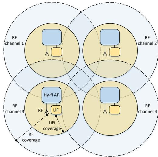
Figure 6. Hy-Fi AP placement in dense enterprise deployments. While adjacent AP use different RF channels, the LiFi channel is the same for all APs as the LiFi cells are non-overlapping.
