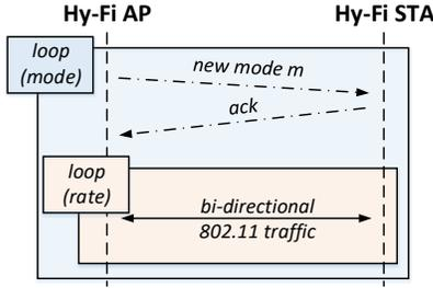
Figure 4. The  $\text{Hy-Fi-AP}$  performs joint mode and rate control. Any mode change is signaled towards the corresponding STA.
