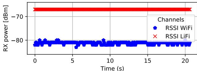
Figure 23.  $H_{y-Fi}$  under continuous jamming on the RF channel with proposed interference management scheme.
