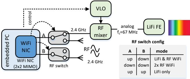
Figure 2.  $H_{y-Fi}$  transceiver design for aggregated LiFi and WiFi.
