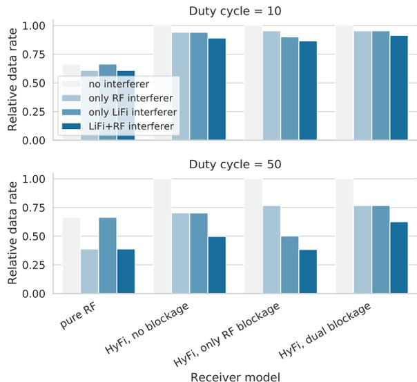
Figure 14. Relative data rate for different receiver and interferer models for the duty cycles 10%, and 50%.
