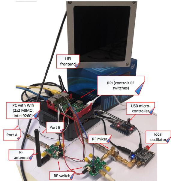
Figure 11.  $H_Y\text{-}F_i$  prototype (AP+STA).
