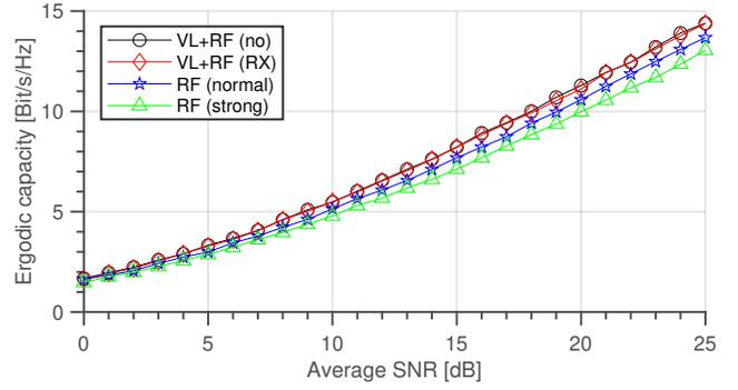
Figure 9. Ergodic MIMO channel capacity.
