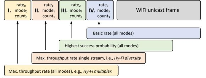
Figure 5. Transmission descriptor set for MRR chain adapted for  $\text{Hy-Fi}$ .
