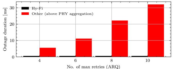
Figure 16. Outage duration in case of sudden blockage of the LiFi channel when operating in the multiplexing mode.
