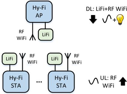
Figure 1. Envisioned scenario with aggregated LiFi plus RF WiFi channel used in the downlink.
