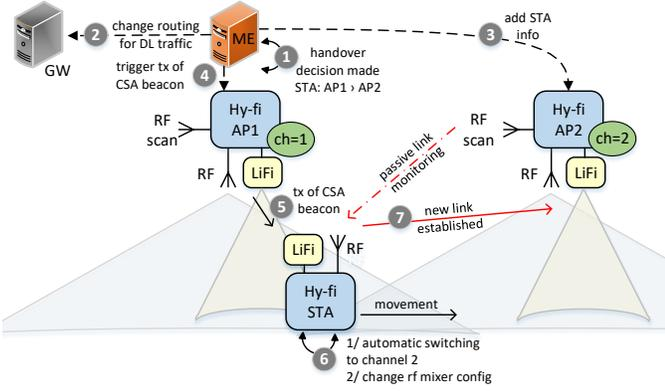
Figure 8.  $\text{Hy-Fi}$  handover operation triggered by the infrastructure: client STA is moved from AP1 to AP2.
