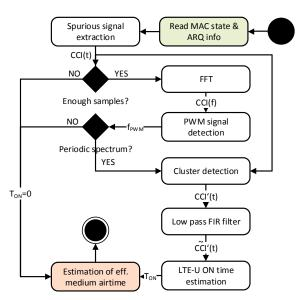
Fig. 6: Flow chart of LTE-U duty cycle detector.
