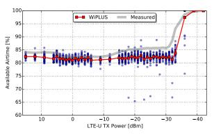
Fig. 10: WiPLUS results for LTE-U BS with CSAT cycle length of 160 ms.
