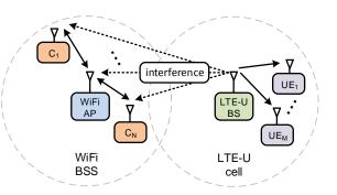
Fig. 3: System model — WiFi BSS co-located with LTE-U cell. The LTE-U DL traffic creates interference on WiFi BSS DL and uplink (UL) traffic.
