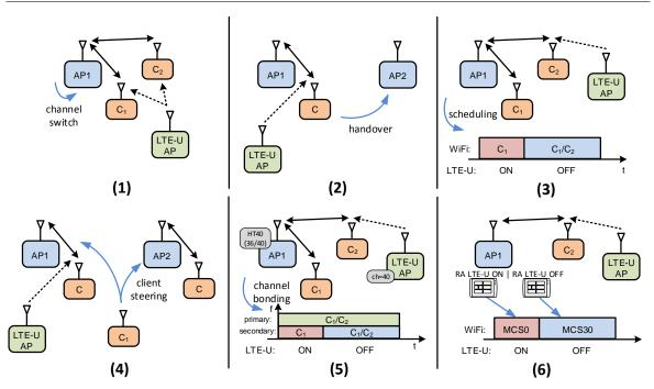
Fig. 8: WiPLUS apps: (1) Interference-aware Channel Assignment, (2) Interference-aware Load Balancing Clients, (3) Interference-aware Medium Access, (4) Interference-aware Client Association Steering, (5) Interference-aware Channel Bonding, (6) Interference-aware Rate Adaptation.
