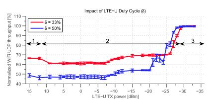
Fig. 1 shows results of our own experiments in which a single high quality WiFi link was suffering from interferrence of a LTE-U Base Station (BS). In particular the normalized UDP throughput of the WiFi link under LTE-U interference, relative to the noninterfered WiFi link, which corresponds to the effective available medium airtime, as a function of different interfering signal strengths and LTE-U dutycycles, is presented. We can clearly see the impact of the LTE-U duty cycle on the WiFi
