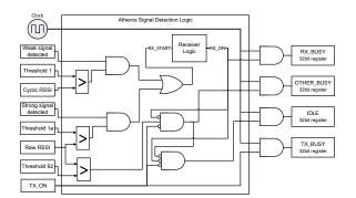
Fig. 7: Block diagram of Atheros signal detection logic and MAC state registers (adapted from [10]).
