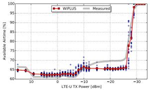
even at very low LTE-U TX power levels, i.e. -29 dBm. For high-power interference, i.e. above ED-CS, the WiFi AP is able to sense the LTE-U signal and the WiFi throughput is reduced (relative to its LTE-U free throughput) by 33% which corresponds to effective time-sharing. At lower LTE-U inteference levels there is a reduction in available medium airtime due to corruption of WiFi packets which again is precisely estimated by WiPLUS. The overall RMSE is around 2.7 percentage points.
