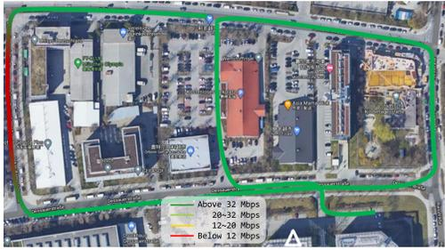
**Fig. 1:** Driving route and uplink throughput of Link Profile 5. The base station is located at  $\blacktriangle$ . The height of the base station antenna is 21 meters above ground level, whereas the vehicle antenna is at approximately 1.5 meter height, mounted on the vehicle roof. The test vehicle traversed the double loop shown by the overlay 10 times.
