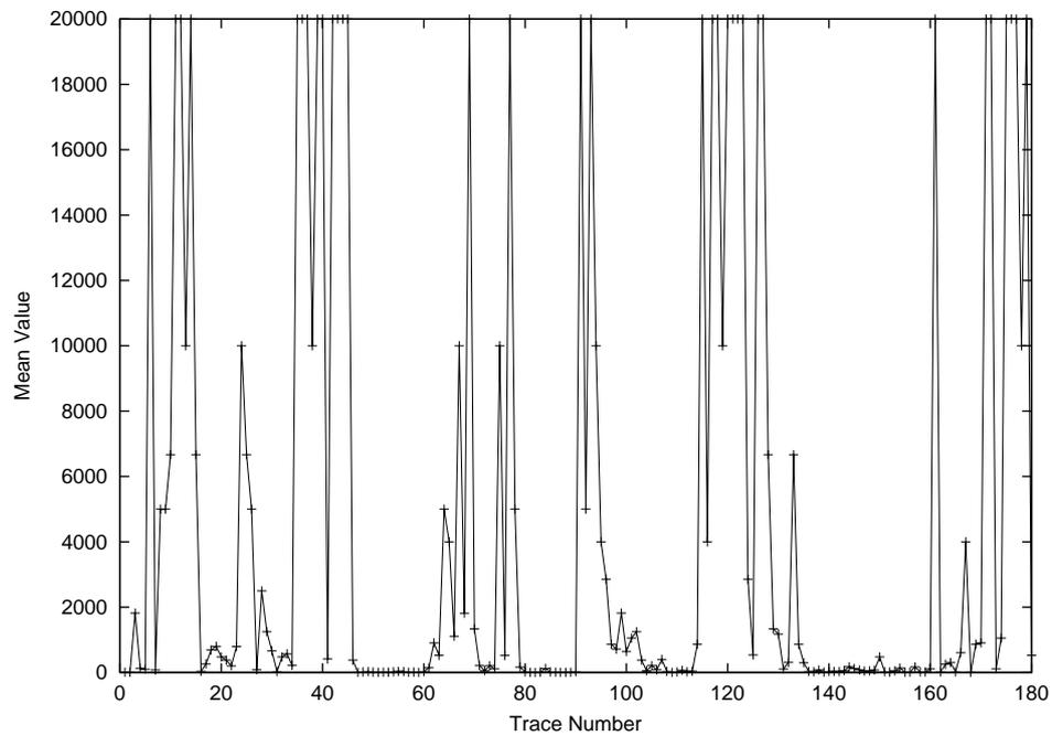
Figure 3.10: Mean packet loss free burst lengths vs. trace number for **longterm1** measurement and burst order  $k_0 = 1$ .
