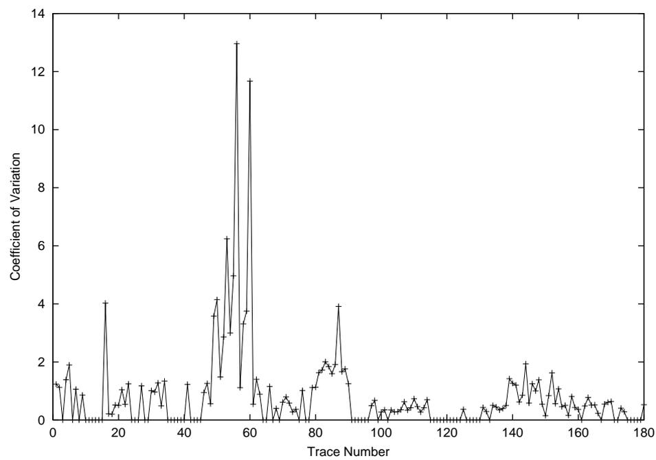
Figure 3.11: Coefficient of Variation of packet loss burst lengths vs. trace number for **longterm1** measurement and burst order  $k_0 = 1$ .
