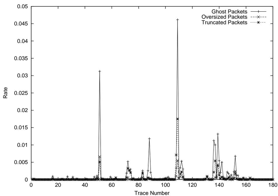
Figure 3.3: Rates of ghost packets, oversized packets and truncated packets vs. trace number for **longterm1** measurement
