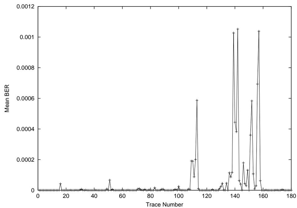
Figure 3.8: Mean bit error rates vs. trace number for **longterm1** measurement (nonlogarithmic scale)
