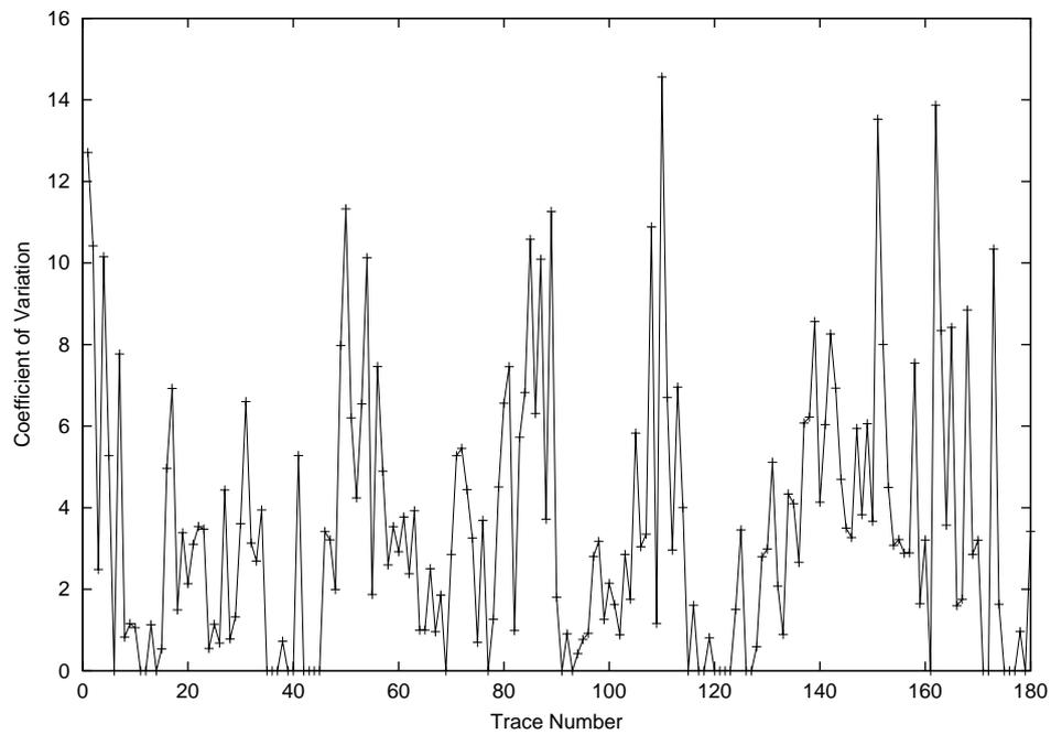
Figure 3.12: Coefficient of Variation of packet loss free burst lengths vs. trace number for **longterm1** measurement and burst order  $k_0 = 1$ .
