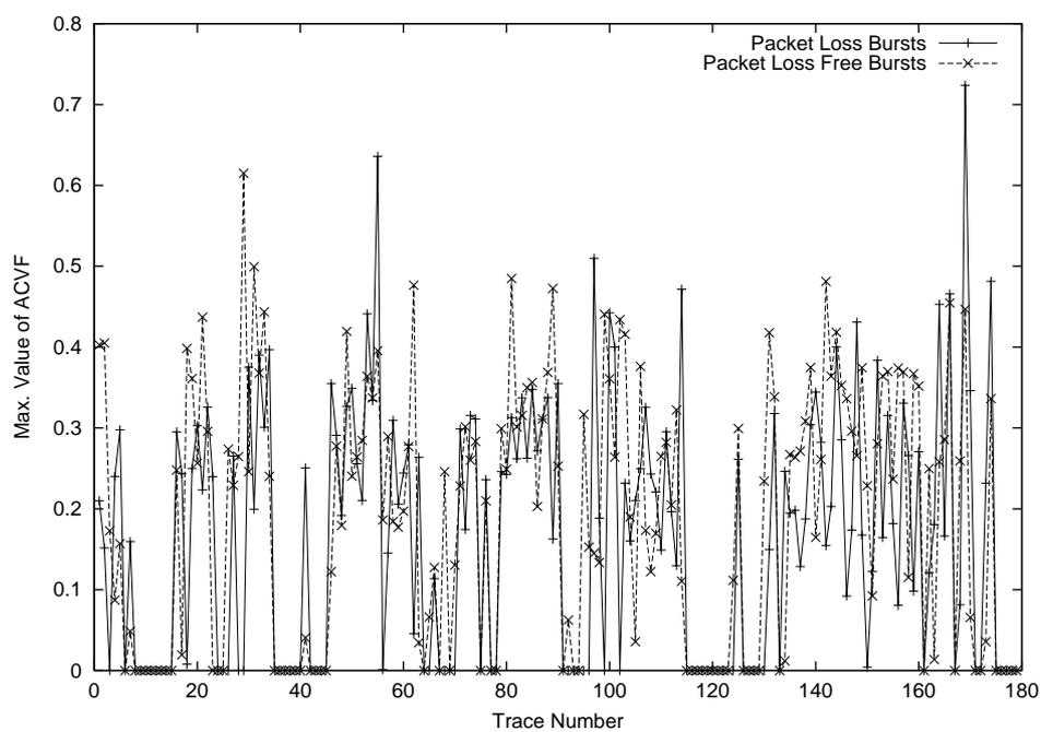
Figure 3.13: Max. values of autocovariance function for packet loss burst lengths and packet loss free burst lengths vs. trace number for **longterm1** measurement and  $k_0 = 1$ .
