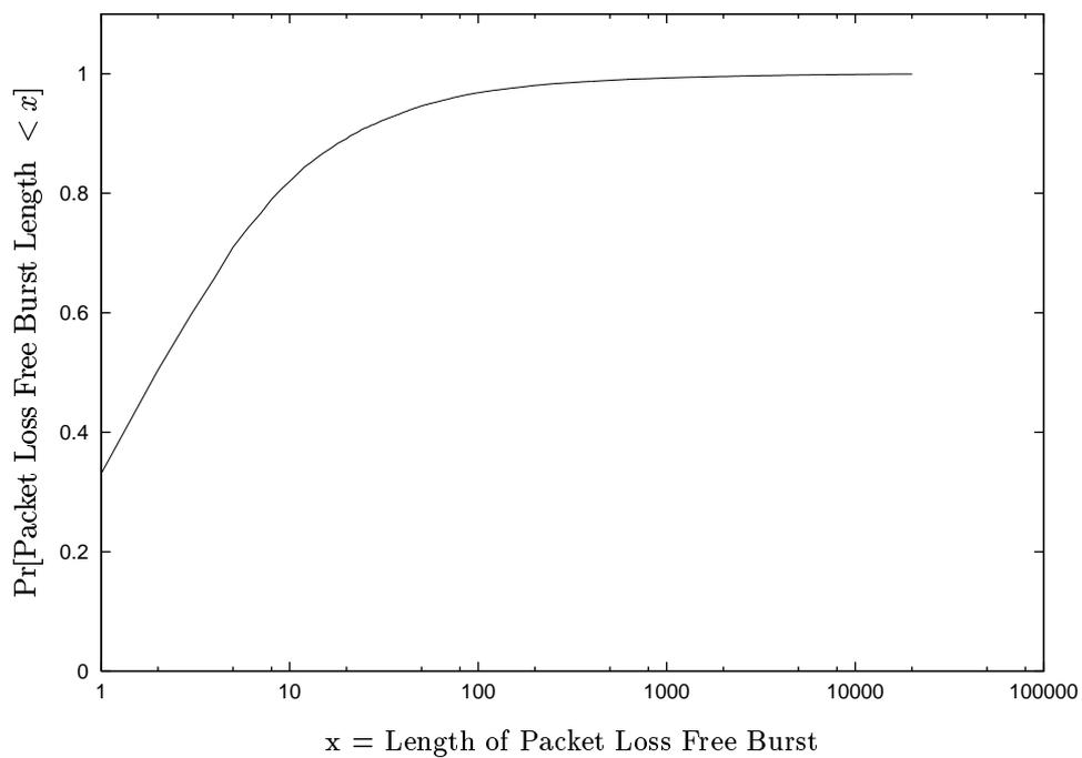
Figure 3.15: Cumulative distribution function of packet loss free burst lengths for compound trace for **longterm1** measurement and  $k_0 = 1$
