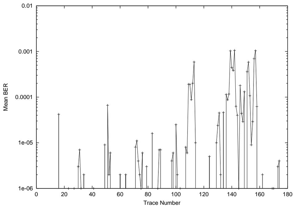
Figure 3.7: Mean bit error rates vs. trace number for **longterm1** measurement
