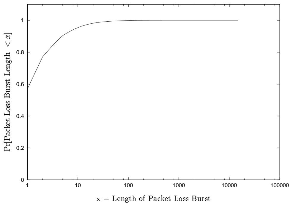
Figure 3.14: Cumulative Distribution Function of packet loss burst lengths for compound trace for **longterm1** measurement and  $k_0 = 1$
