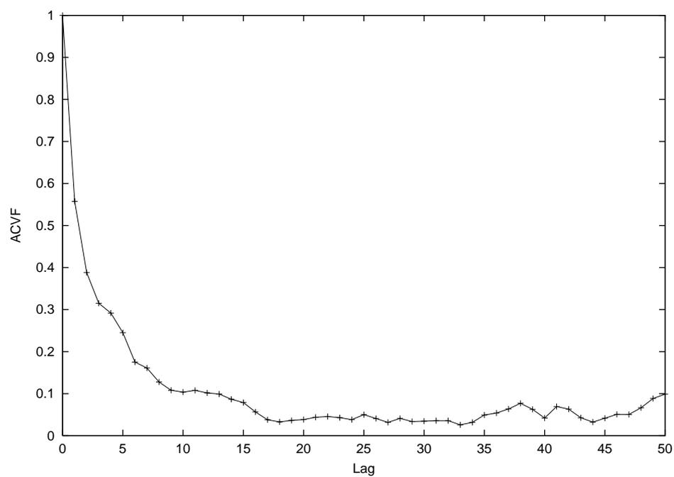
Figure 3.17: Autocovariance function of packet loss free burst length sequence for the compound trace and  $k_0 = 1$  for **longterm1** measurement
