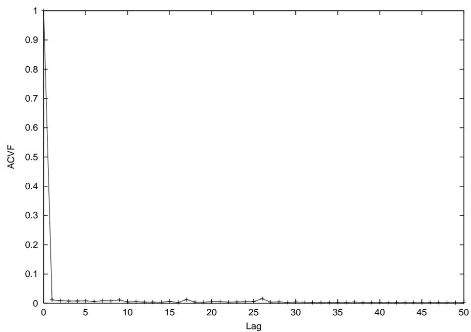
Figure 3.16: Autocovariance function of packet loss burst length sequence for the compound trace and  $k_0 = 1$  for **longterm1** measurement
