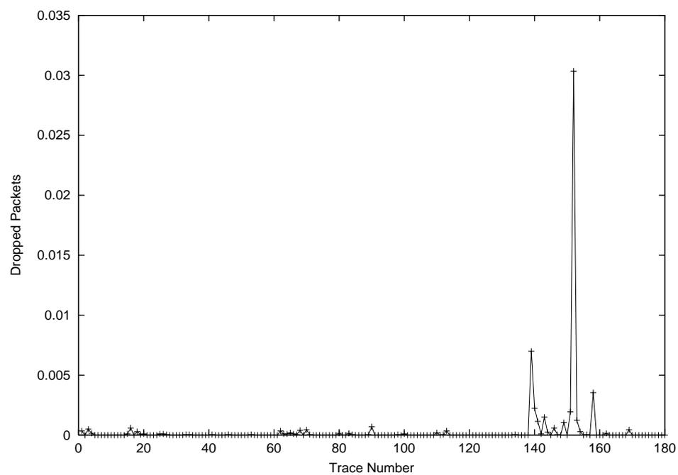
Figure 3.5: Rate of packets dropped due to more than 10% erroneous bits vs. trace number for **longterm1** measurement
