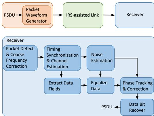
Fig. 9: Block diagram for the implemented transmission-reception scheme according to the 802.11ad.
