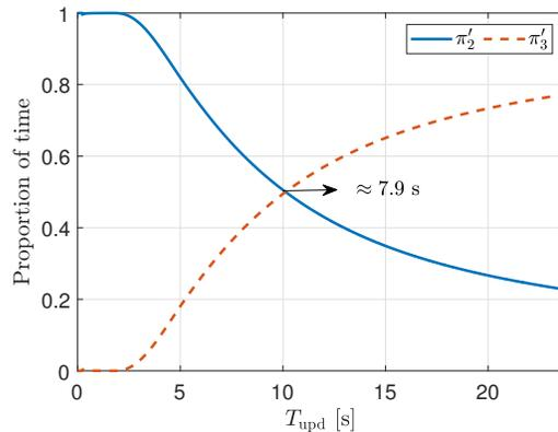
Fig. 12: Fraction of time in the inner and outer areas when  $r_{in} = 1.7$  m,  $r_{out} = 3$  m,  $v = 1$  m/s.
