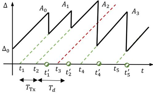
Fig. 7: Illustration of the AoI of packets (dashed lines) and as perceived on a given destination node (bold line).
