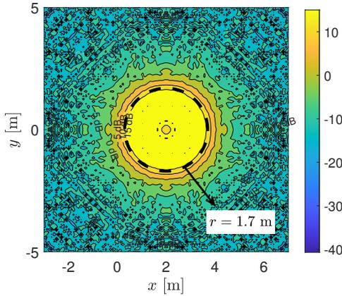
Fig. 10: Heat map of the SNR values for the IRS's illuminated area and the parameters given in Table I, following the framework presented in [28].
