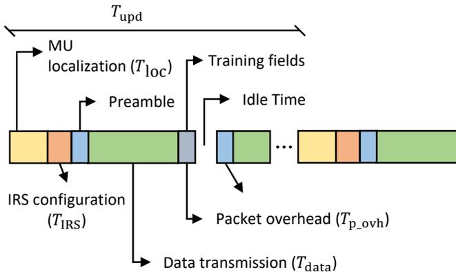
Fig. 2: Frame structure for IRS-assisted downlink transmission [29].
