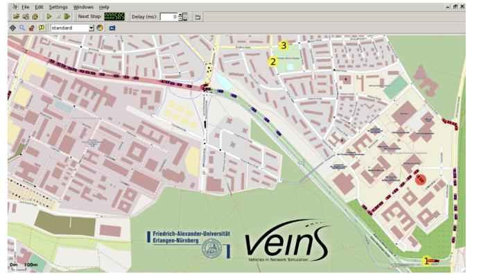
Fig. 2. Screenshot of the running simulative prototype. A contiguous stream of vehicles, leaving the university campus and heading to a business park, was interrupted by a traffic obstruction at point ①. Dynamic re-routing has started.
