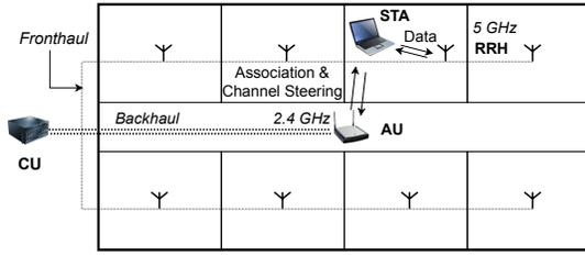
Figure 3. Example Ce-Fi deployment with RRHs in each room, connected to the CU via a packet FH, and with a centrally located AU connected to the CU via a backhaul.
