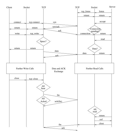
Figure 4.2.: Example communication scenario using the socket interface
