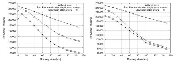
(a) Loss occur after link capacity is reached
