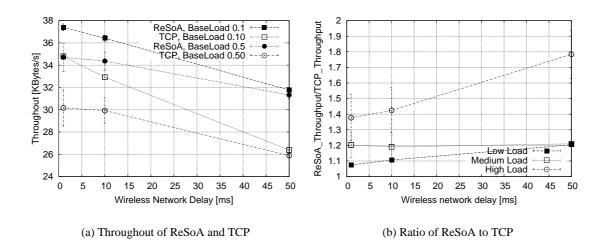
Figure 10.27.: Effects of background traffic on the performance of ReSoA and TCP as a function of wireless network delay. Wireless network bitrate 384kb/s, Internet bitrate 2Mb, Internet delay 40ms
