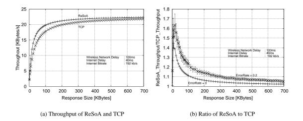
Figure 10.12.: ReSoA vs. TCP for a wireless network bitrate of 384kb/s as a function of the response size.
