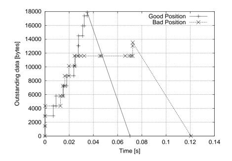
Figure 9.7.: Outstanding data at Good- and Bad-Position for end-to-end TCP
