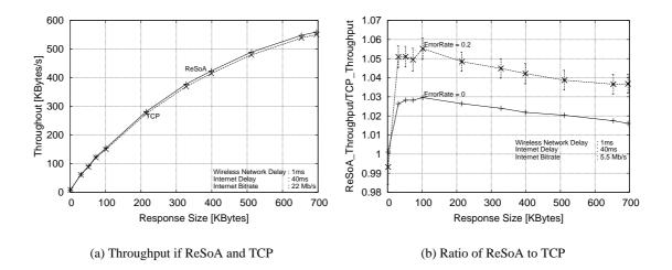
Figure 10.21.: ReSoA vs. TCP for a wireless network bitrate of 11Mb/s as a function of the response size
