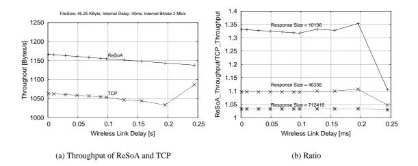
Figure 10.9.: TCP vs. ReSoA as a function of the wireless network delay. Parameter: No erros, wireless bitrate 9600 bits/s, Internet delay: 40 ms, Internet bitrate: 2Mb/s
