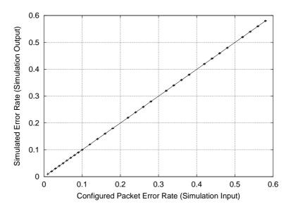
Figure D.1.: Test of the uniform error model. The bitrate was set to 1 Mb/s and the packet size was 1000 Bytes. The simulation time was 500 seconds. The plot shows the mean observed packet error rate and a 95% confidence level.
