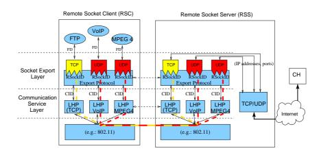
Figure 5.2.: Basic components of ReSoA
