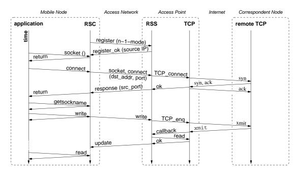
Figure 5.3.: Example message exchange resulting from an application using a ReSoA-client and a ReSoA-server configuration to access the Internet
