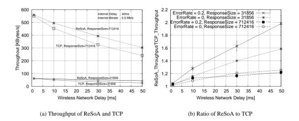
Figure 10.22.: ReSoA vs. TCP for a wireless network bitrate of 11Mb/s as a function of the wireless network delay
