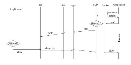
Figure 6.10.: shutdown-call on corresponding host when wireless host uses ReSoA
