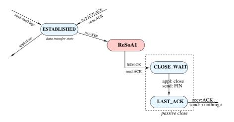
Figure 6.16.: Modification number 1 to TCP state transistion diagram
