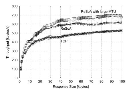
Figure 9.3.: ReSoA versus TCP at the Good-Position. The figure shows the median throughput achieved for different response sizes. The errorbars show the range between the lower and upper quartiles.
