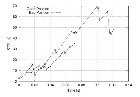
Figure 9.8.: RTT over time at Good- and Bad-Position for end-to-end TCP
