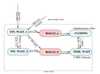
Figure 6.17.: Modification number 2 to TCP state transistion diagram
