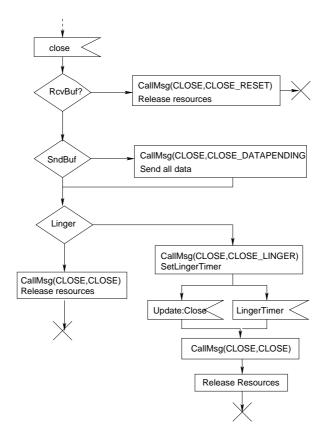
Figure 6.7.: Flow chart of close implementation at the ReSoA-client
