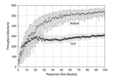
Figure 9.5.: Measurement results for ReSoA versus end-to-end TCP at the Bad-Position. The figure shows the median throughput achieved for different response sizes. The errorbars show the range between the lower and upper quartiles.
