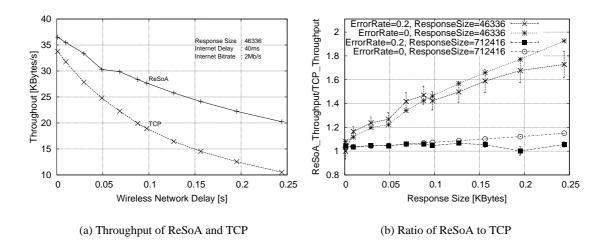
Figure 10.16.: ReSoA vs. TCP as a function of the wireless network delay. The wireless network bitrate was set to 384kb/s.
