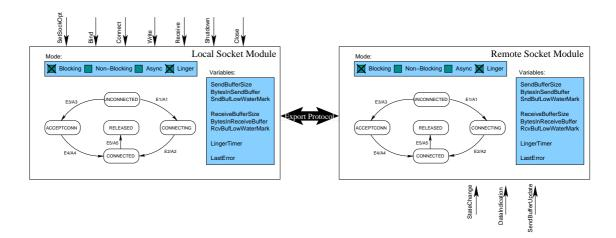
Figure 6.3.: Realization of a socket in ReSoA
