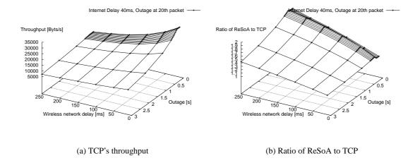
Figure 10.29.: ReSoA vs. TCP in the case of outages and a response size of 50680.
