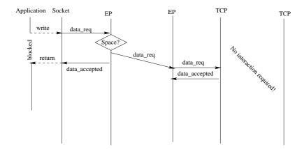
Figure 6.15.: write-call: version 4 - using ReSoA
