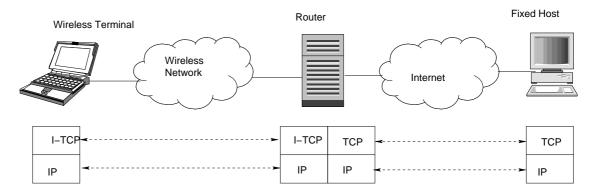
Figure 3.4.: The principle of transport protocol splitting
