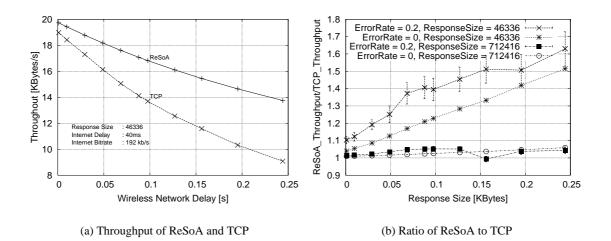
Figure 10.13.: ReSoA vs. TCP for a wireless network bitrate of 384kb/s as a function of the wireless network delay
