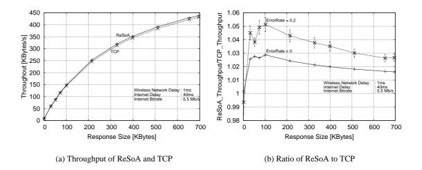
Figure 10.18.: ReSoA vs. TCP for a wireless network bitrate of 11Mb/s as a function of the response size
