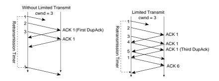
Figure 2.4.: Limited Transmit example
