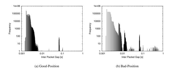
Figure 9.2.: Rating of Good- and Bad-Position using the inter-packet gap of a UDP flow
