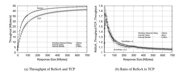
Figure 10.15.: ReSoA vs. TCP for a wireless network bitrate of 384kb/s as a function of the response size.
