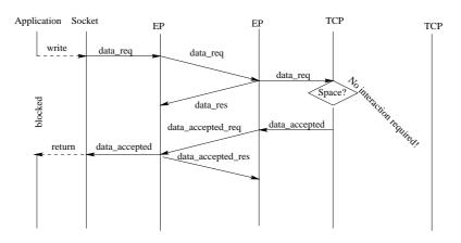
Figure 6.12.: write-call: version 1 using ReSoA
