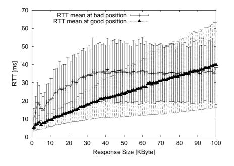
Figure 9.6.: Mean RTT and standard deviation at Good- and Bad-Position for end-to-end TCP.
