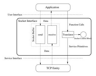
Figure 4.1.: Basic components and interfaces of a socket
