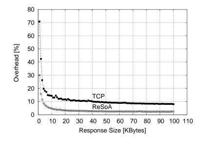
Figure 9.4.: ReSoA vs. TCP at the Good-Position. The figure shows the mean overhead of ReSoA and TCP as a function of the response size.
