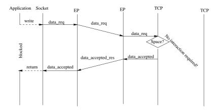
Figure 6.13.: write-call: version 2 - using ReSoA
