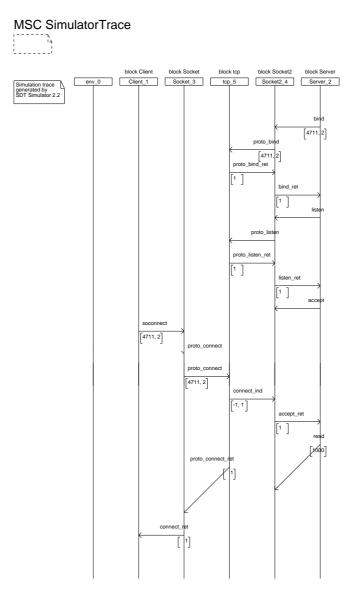
Figure B.1.: MSC: Connection establishment using BSD socket
