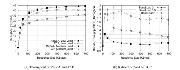
Figure 10.26.: Effects of background traffic on the performance of ReSoA and TCP as a function of the response size. Wireless network bitrate 384 kb/s, Wireless network delay 50ms, Internet bitrate 2 Mb, Internet delay 40 ms
