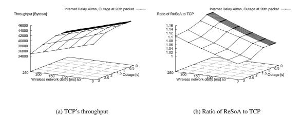
Figure 10.30.: ReSoA vs. TCP in the case of outages and a response size of 709520 bytes.
