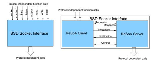
Figure 6.1.: Splitting the socket interface
