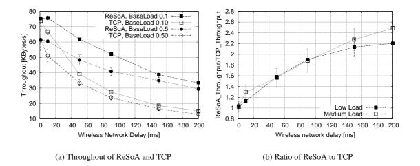
Figure 10.25.: Effects of background traffic on the performance of ReSoA and TCP as a function of wireless network delay. Wireless network bitrate 11Mb/s, Internet bitrate 2Mb, Internet delay 40ms
