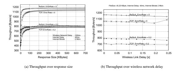
Figure 10.10.: TCP's and ReSoA's throughput in the case of uniformly distributed errors and a wireless network bitrate of 9600 b/s
