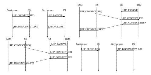
Figure C.2.: LHP service primitives for connection management
