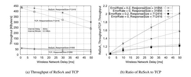
Figure 10.19.: ReSoA vs. TCP for a wireless network bitrate of 11Mb/s as a function of the wireless network delay
