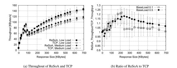
Figure 10.24.: Effects of background traffic on the performance of ReSoA and TCP as a function of the response size. Wireless network bitrate 11Mb/s, wireless network delay 1ms, Internet bitrate 2Mb/s, Internet delay 40ms
