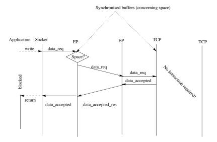
Figure 6.14.: write-call: version 3 - using ReSoA
