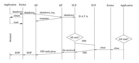
Figure 6.11.: shutdown-call on wireless host using ReSoA
