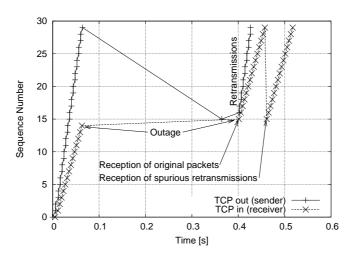
Figure 3.3.: Results of example simulation showing effects of a spurious timeout on the behavior of the TCP sender. The simulated scenario is a file transfer between two directly connected hosts. As file size we have chosen 30 KB arbitrarily. During the transfer we simulated an outage period. The figure shows that no TCP segment is lost (every segment sent is received by the receiver) and that, in spite of this, the TCP sender enters retransmit mode performing Go-Back-N.
