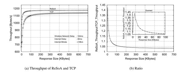
Figure 10.8.: TCP vs. ReSoA over response size. Parameters: No errors, wireless link delay: 100ms, Internet delay: 40ms, wireless bitrate 9600b/s, Internet bitrate: 2Mb/s
