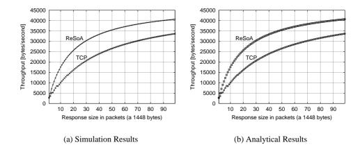
Figure 10.6.: Comparison of analytical results and simulation results. The set-up consists of a two hop network. The client and the router (ReSoA-server) are connected by a full-duplex link with 384Kb and 100ms latency one way. The server is connected to the router (ReSoA-server) by a second full-duplex link with 100Mb and 25ms latency one way. No packets were lost. We show the simulation results and analytical results in different figures since the curves are congruent.
