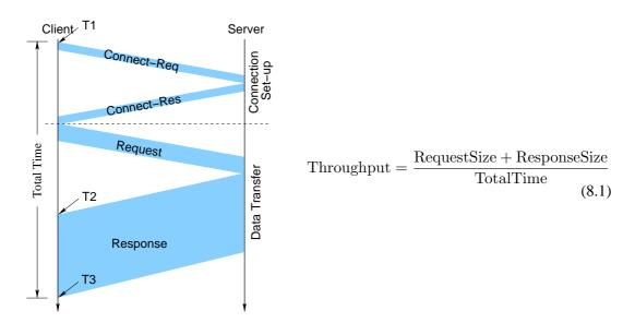
Figure 8.1.: Communication scenario and definition of the metric used for the performance evaluation
