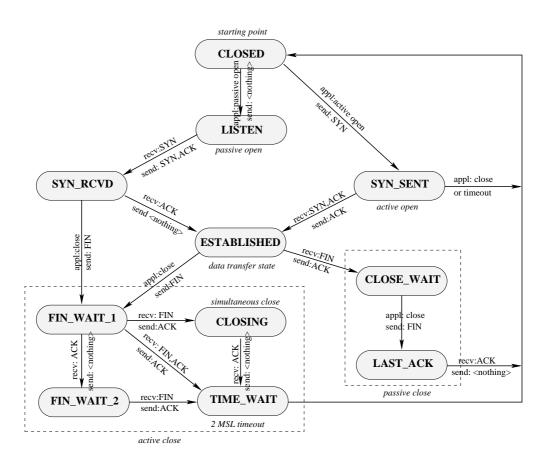
Figure 2.2.: TCP state transition diagram
