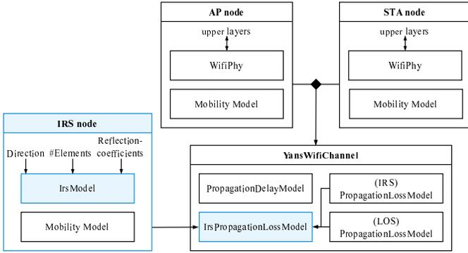
Figure 2: Architecture of ns3IRS; we introduce IRS node and IRSPropagationLossModel classes.
