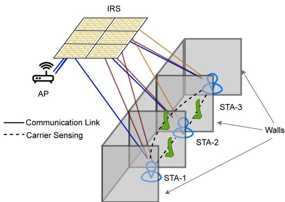
(a) *P1: Centralized IRS*: Further splitting the IRS such that it creates connectivity between the STAs.
