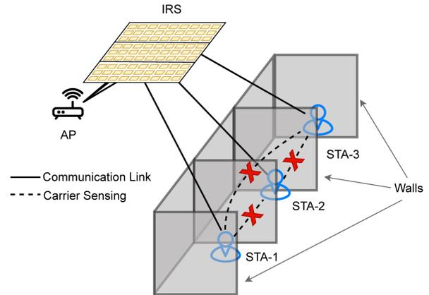
Figure 1: An IRS is used to enable/improve the communication links between the AP and the STAs. Here a single IRS is split into multiple tiles so that each tile is optimized for a particular AP-STA link. This may lead to the creation of hidden terminals.
