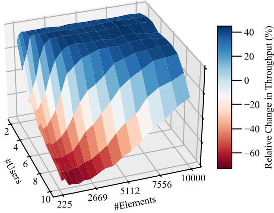
Figure 5: Relative throughput increase of *P1: Centralized IRS* in comparison to CSMA/CA with RTS/CTS baseline (*BL2: RTS/CTS*) depending on IRS size.
