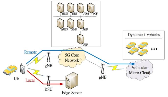
Figure 1. Proposed offloading system architecture
