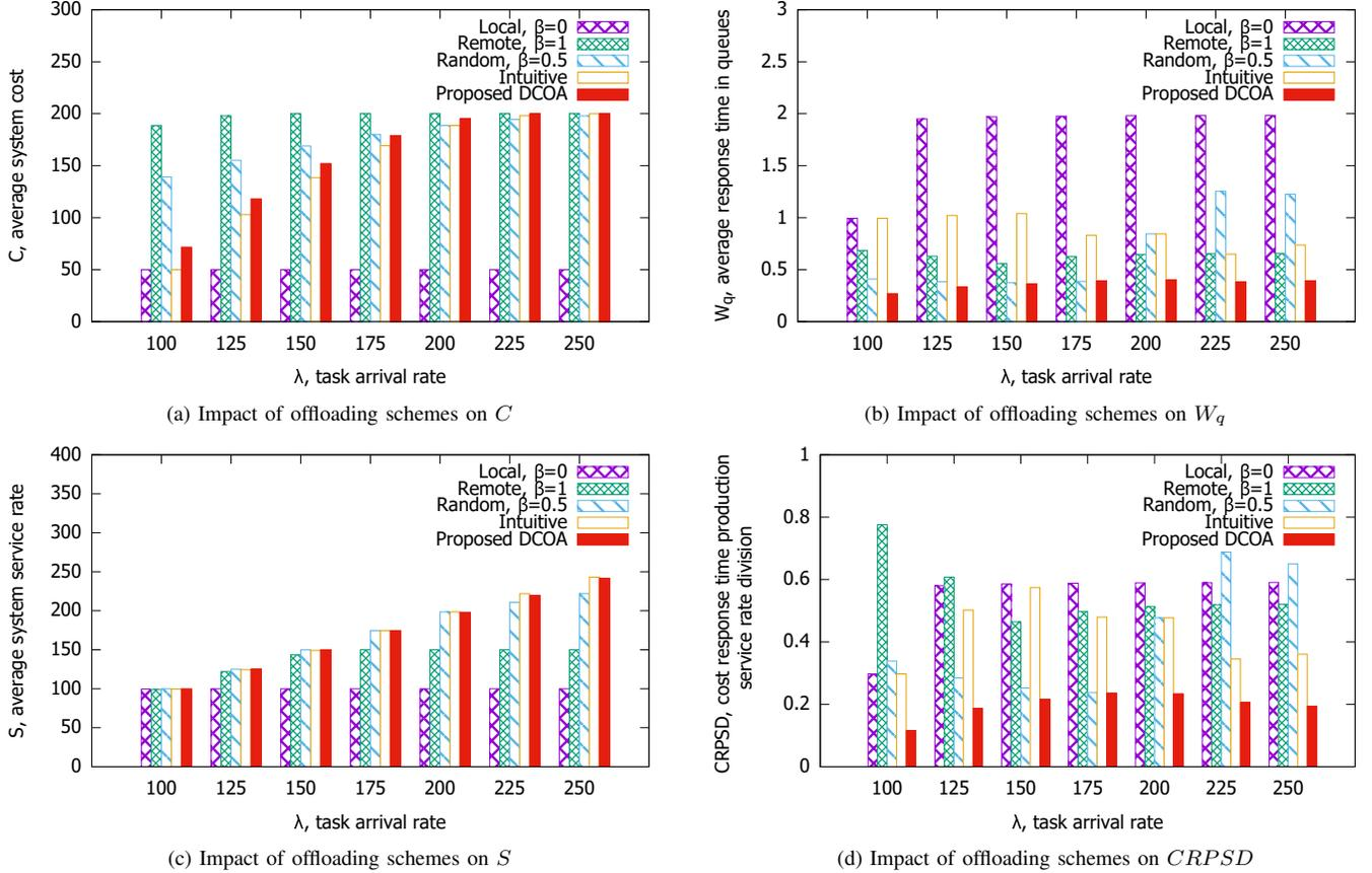
Figure 3. Impact of offloading schemes
