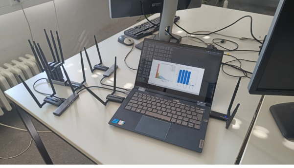
Figure 3. The PDF-WiN prototype with 802.11ax NICs connected via USB.
