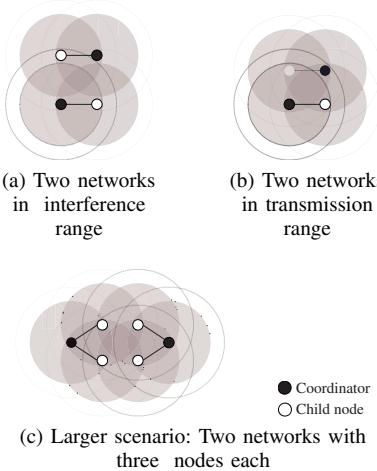
Figure 2: Simulation scenarios for co-located WPANs
