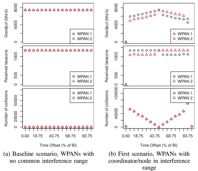
Figure 4: Simulation results: not in communication range
