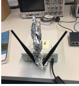
Figure 4: Experimental setup showing USRP device and aluminium foil between its transmit and receive antenna for passive SI suppression.
