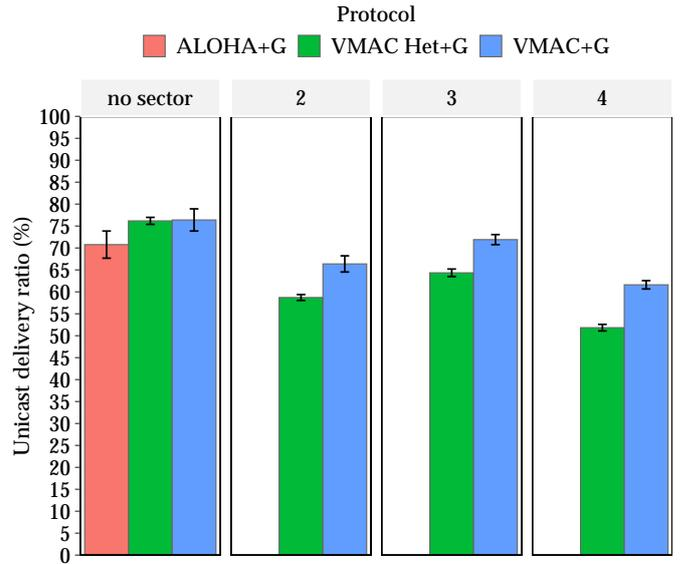
Figure 12: Unicast delivery ratio for V-VLC transmissions for VMAC protocols with GPS positions feature. Varying number of sectors is noted above the corresponding plot. ALOHA does not support multiple sector configurations, hence not shown.
