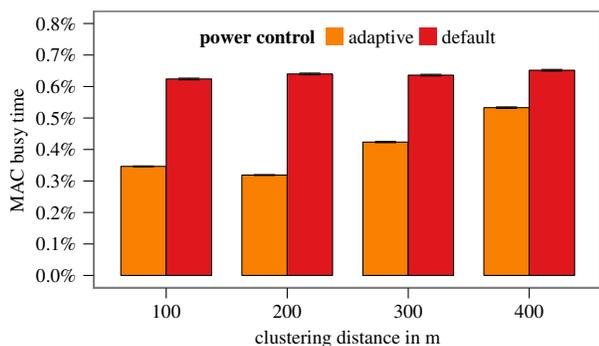
Figure 5. DSRC channel utilization for adapted transmit power vs. default transmit power.
