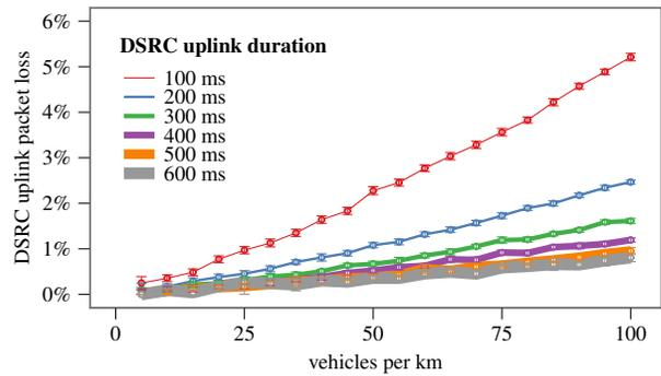
Figure 2. DSRC uplink packet loss for different node densities and interval durations.
