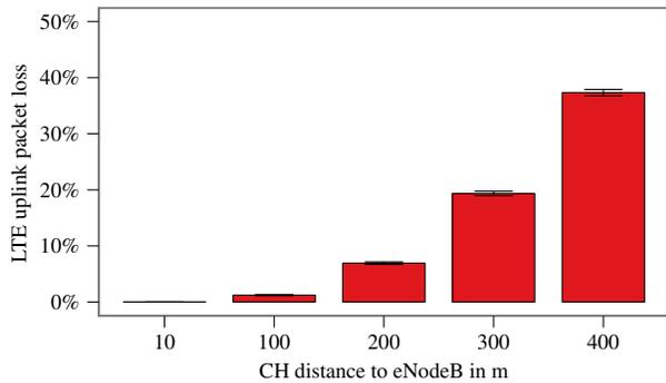
Figure 3. LTE uplink packet loss as a function of the distance between the Cluster Heads (CHs) and the eNodeB.
