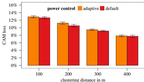
Figure 4. CAM Loss for adapted transmit power vs. default transmit power.
