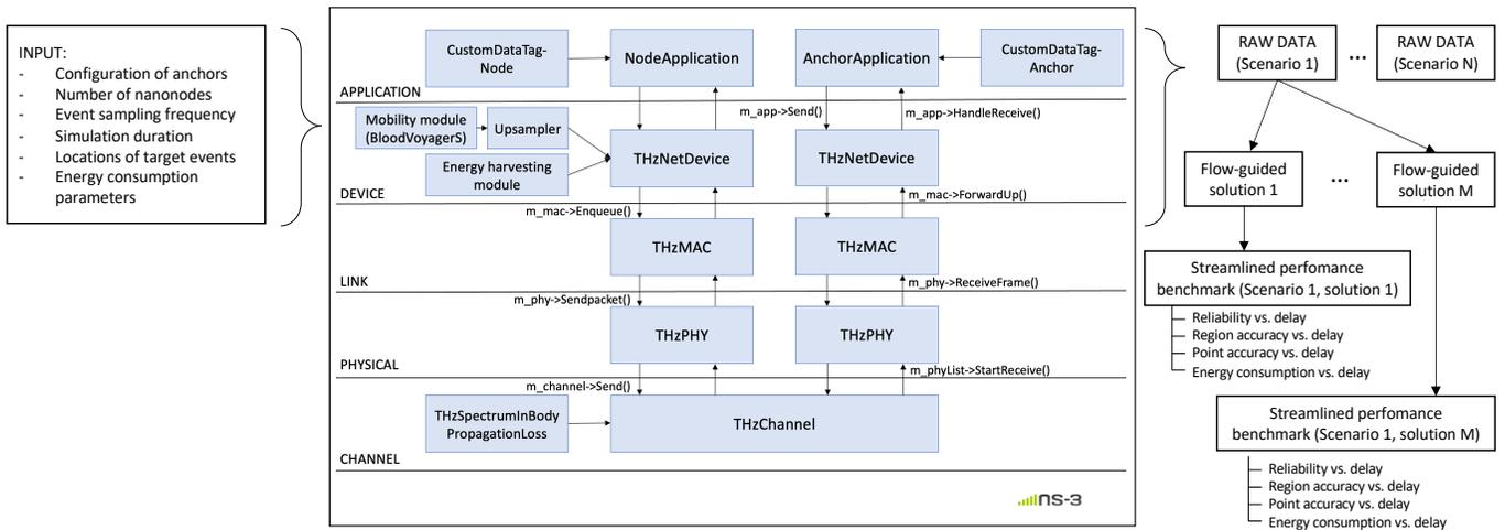
Figure 4. Overview of the framework for standardized performance evaluation of flow-guided localization
