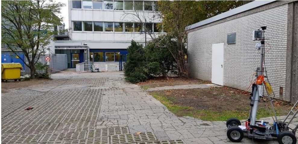
Figure 24 – Transition from LOS to NLOS due to foliage. Node 2 at measurement position 13
