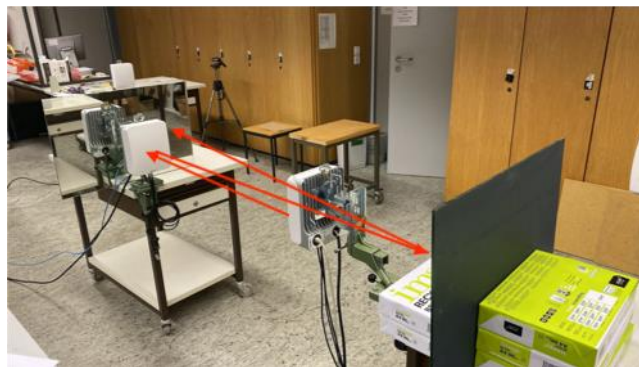
Figure 99 – EXP 5: Short-range LOS with mirrors to create multiple reflections
