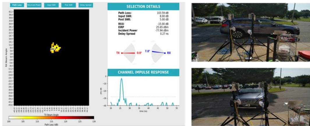
Figure 48 – Car dielectric constant measurements
