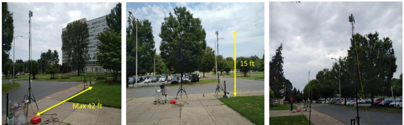
Figure 40 – Outdoor short-distance measurements of path loss
