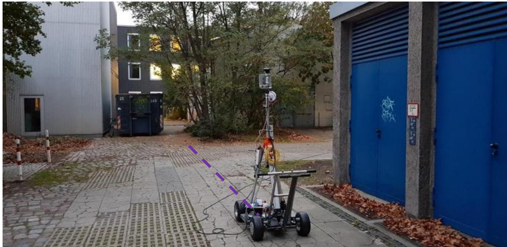
Figure 25 – NLOS scenario due to solid building. Node 2 at measurement position 16
