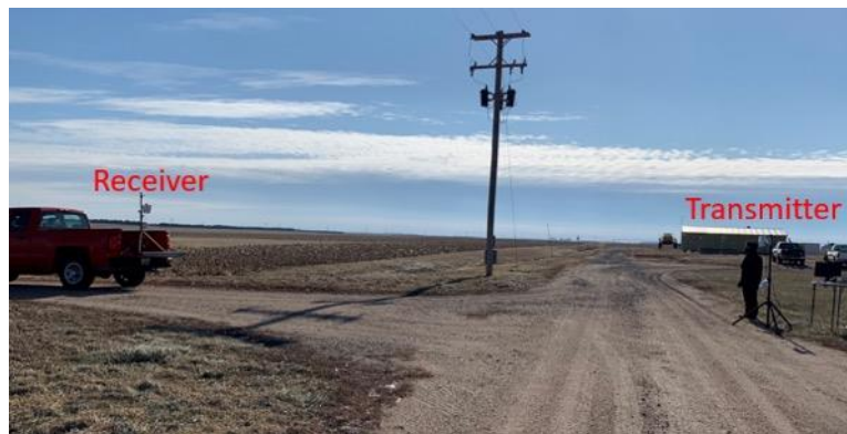
Figure 81 – Tx and Rx setup for the field measurements
