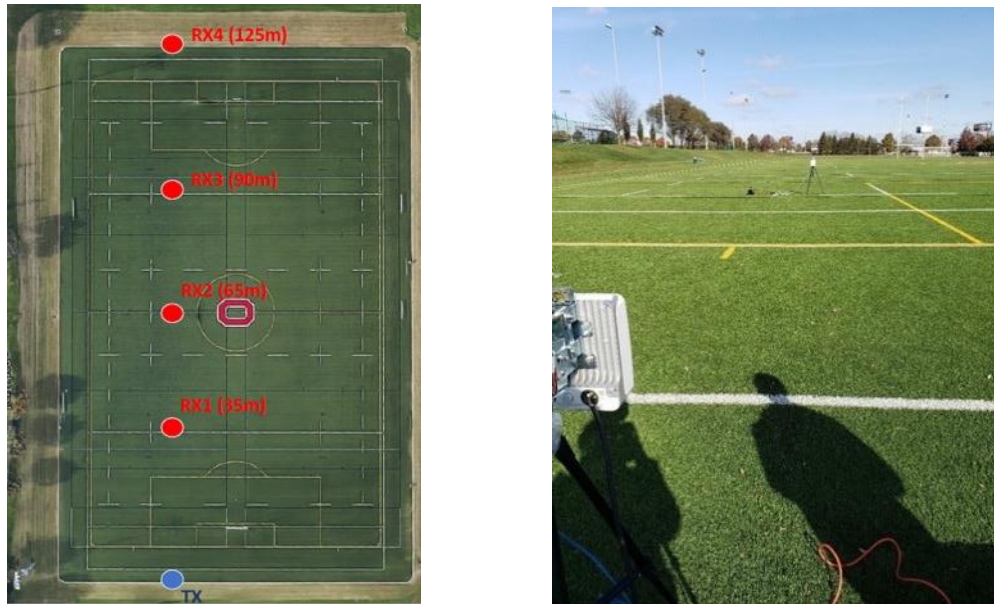
Figure 79 – Outdoor experiments were conducted in a football field by placing Rx at four locations (red circles)
