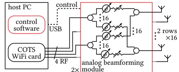
Figure 1: Architecture of the HDA MU-MIMO system with the HDA extension marked in red.
