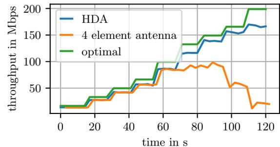
Figure 4: iperf3 throughput of the HDA system and the 4 element antenna system during a MCS sweep.
