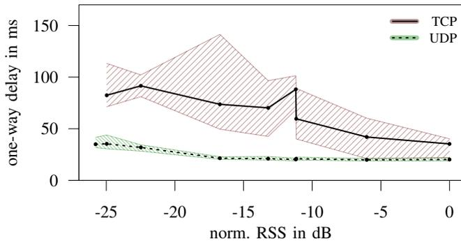
Figure 4. Delay of TCP and UDP traffic in line scenario.
