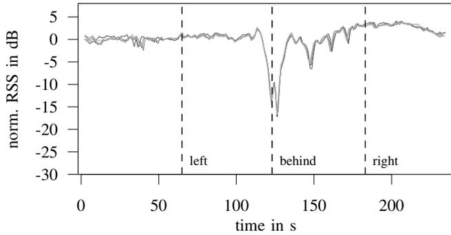
Figure 9. RSS while driving around the forage harvester with the discharge chute elevated.
