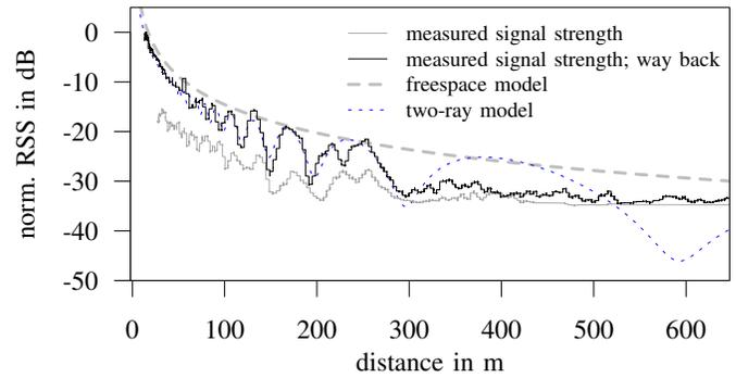
Figure 6. Signal strength of dynamic measurements with reduced transmit power in line scenario.
