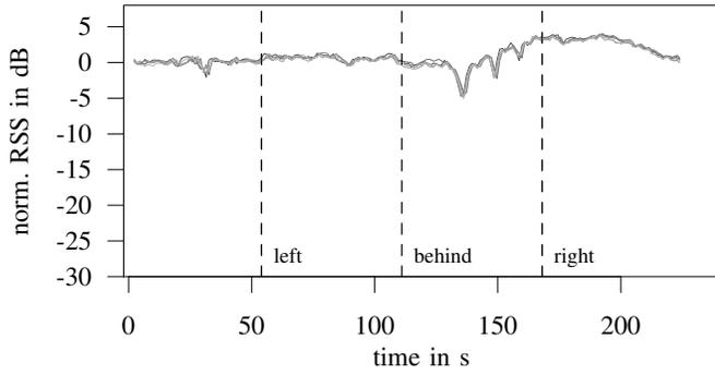
Figure 8. RSS while driving around the forage harvester with the discharge chute at its lowest position.
