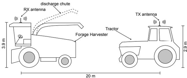
Figure 1. Overview of the used vehicles and the position of the antennas.
