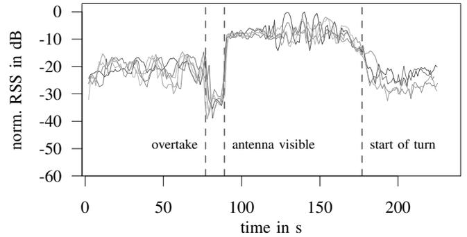
Figure 12. Received signal strength in the harvesting scenario.
