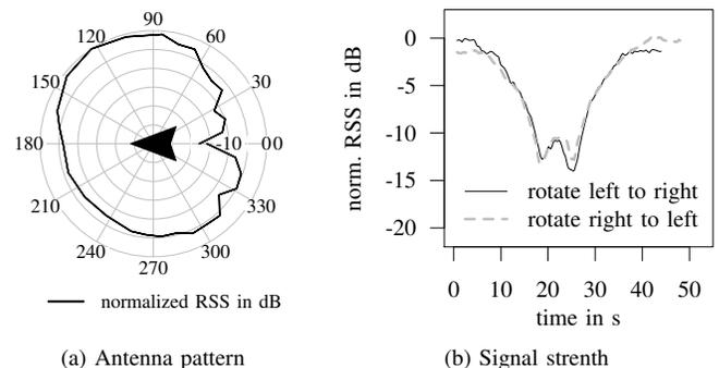
Figure 7. Impact of discharge chute of forage harvester on RSS
