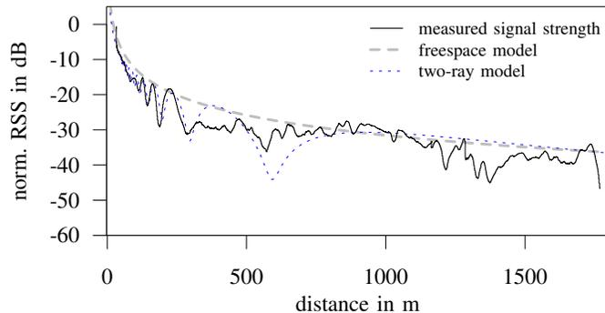
Figure 3. Signal strength of dynamic measurements in line scenario.
