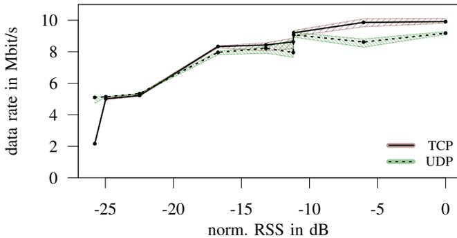
Figure 5. Goodput of TCP and UDP traffic in line scenario.
