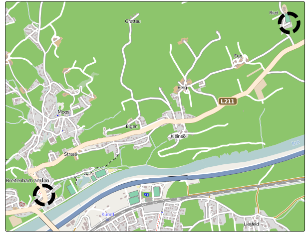
Fig. 3. Scenario modeling the municipality of Breitenbach am Inn/Tirol , as imported from OpenStreetMap. A single traffic flow starts from Ried (top right corner) and is heading to Dorf (bottom left corner). An artificial accident is introduced at a fixed point in time. ATB enables vehicles to calculate and take detours as necessary.
