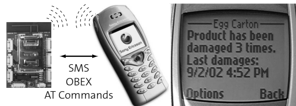
Figure 3. Product monitoring using BTnodes as smart tags and SMS via mobile phones
