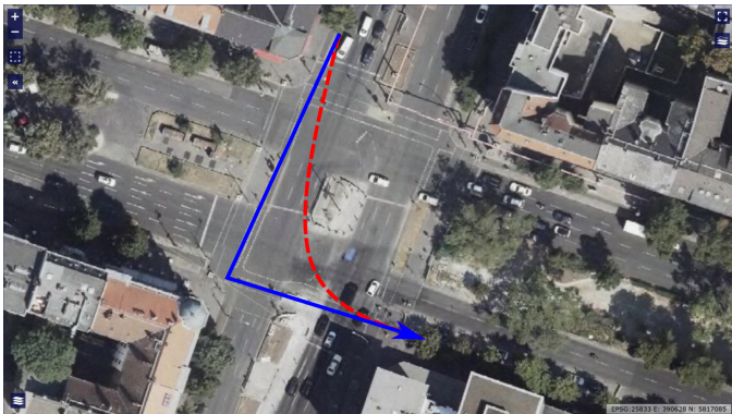
Figure 14: Intersection Mehringdamm/Gneisenaustraße: a traffic island obstructs the direct turn path (dashed line) and, thus, makes the indirect path (solid line) more likely to be used.
