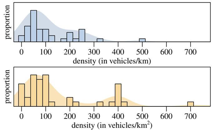
Figure 6. Distribution of used vehicle densities (top: highway, bottom: urban).
