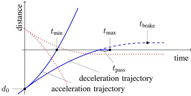
Fig. 2. Graphical derivation of  $t_{\min}$  and  $t_{\max}$ . All labels and variables refer to solid blue line (first car), mirrored w.r.t.  $x$  axis for clarity. The second car is represented by the dotted red line.
