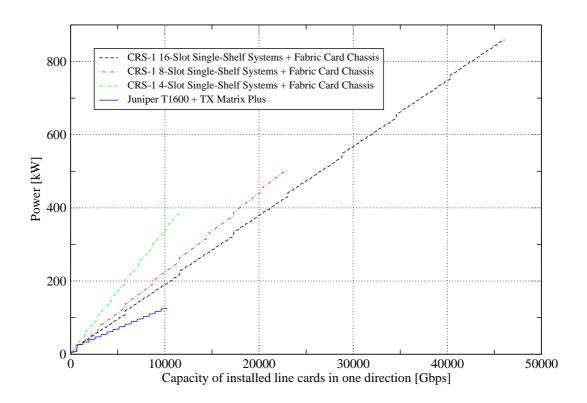
Figure 1: Router power consumption versus capacity (as unidirectional capacity of installed 40 Gbps OC-768c/STM-256c line cards) for Cisco CRS-1 single and multi shelf systems as well as Juniper T1600 interconnected by Juniper TX Matrix Plus
