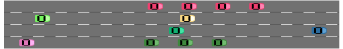
Figure 1. Screenshot from the Sumo-based live GUI of PlaFoSim: a freeway with 4 lanes, many individual vehicles, and 2 platoons.
