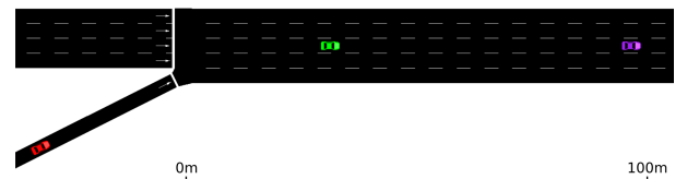
Figure 2. Screenshot of the simulation scenario. The red car is approaching the entrance ramp of the freeway while two other cars are performing a join maneuver (the green car is joining the purple one).
