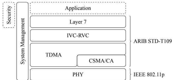
Figure 1. The protocol stack of ARIB STD-T109. Dashed lines indicate entities which are out of the scope of the standard.
