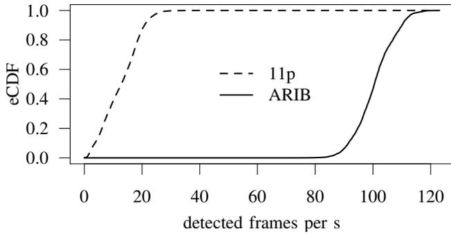
Figure 8. The total number of detected frames ARIB T109 in comparison to IEEE 802.11p.
