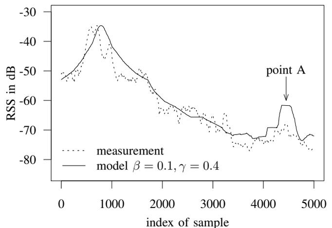
Figure 5. The received signal strength for 868 MHz fitted to the analytical model. At point A we see the increased signal strength due to the LOS corridor.
