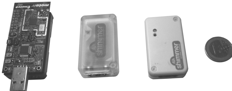
Figure 3.2: WBAN platforms (from left to right): Tmote Sky, Shimmer2 and Shimmer2r.
