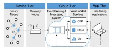
Fig. 1. General architecture of a cloud-centric IoT platform with cloud-based message bus and value-added services.
