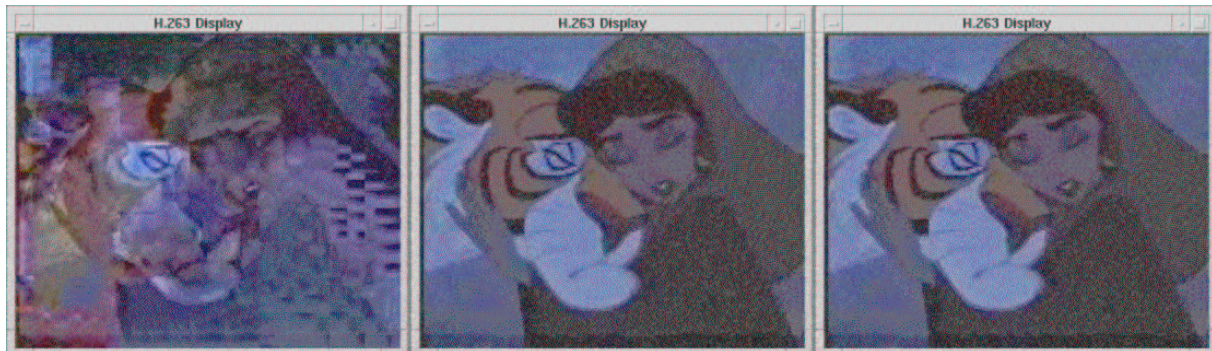
Figure 5.19: Comparison I of video sequence Aladdin after sequential (left), SMPT (middle), and the error-free (right) transmission.
