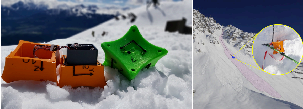
Figure 1: Measurement methods (AvaNodes): Sensor in the field set-up and the outline of an avalanche experiment (light pink) with the estimated trajectory of the particle and the deposition point, as well as the AvaNodes in the avalanche deposit.
