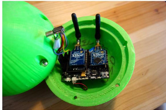
Figure 2: Prototype sample of our 3D printed spheres with the Waspnote sensor node that has a Decawave ToF ranging module and two radios attached
