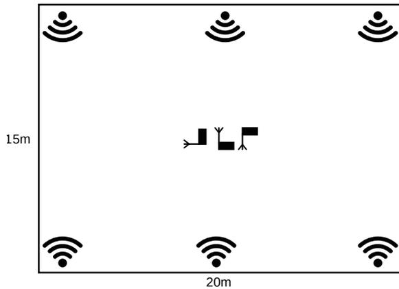
Figure 3: Sketch of the snow test field for the RSS tests: the senders were buried along the outside of the snow field and the receivers were placed in the middle of the area
