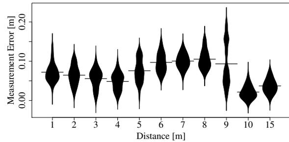
Figure 4: ToF measurement results in line of sight conditions; the horizontal lines show the mean value (Erlacher et al., 2016)
