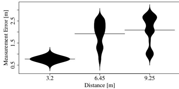
Figure 5: ToF measurement results with sender and receiver buried in snow; the horizontal lines show the mean value
