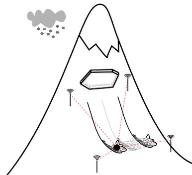
Figure 1: The AvaRange approach: Sensor nodes in robust housings matching the size and density of snow lumps are distributed in the avalanche area and travel together with the avalanche to the run-out.
