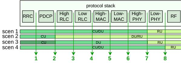
Fig. 5. Functional Splitting and use-case examples.
