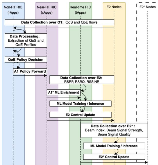
Fig. 10. Information Flow of Multi-Level Control Loops
