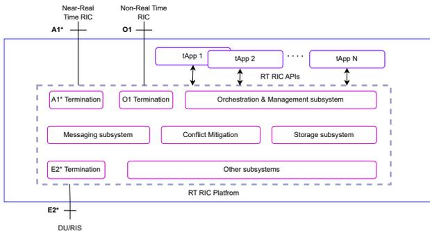
Fig. 7. Real Time RIC architecture.
