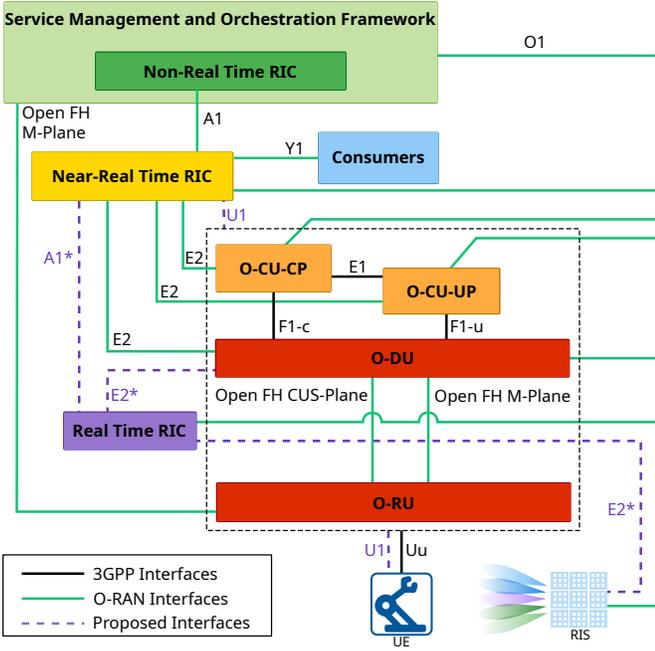
Fig. 6. Proposed extensions to the O-RAN architecture.
