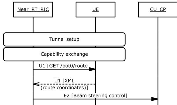
Fig. 8. Route based beam steering using U1.
