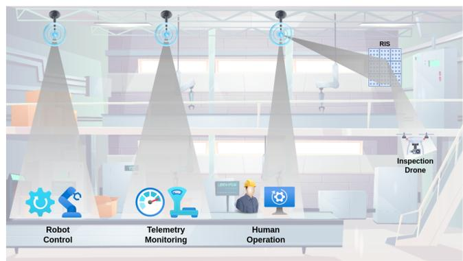
Fig. 2. Smart factory schematic, where multiple radio units (RU) connect to a variety of fixed and mobile devices (UE) either directly or via a reconfigurable intelligent surface (RIS).
