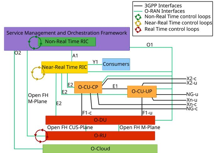
Fig. 4. Based on O-RAN Architecture Description 8.0
