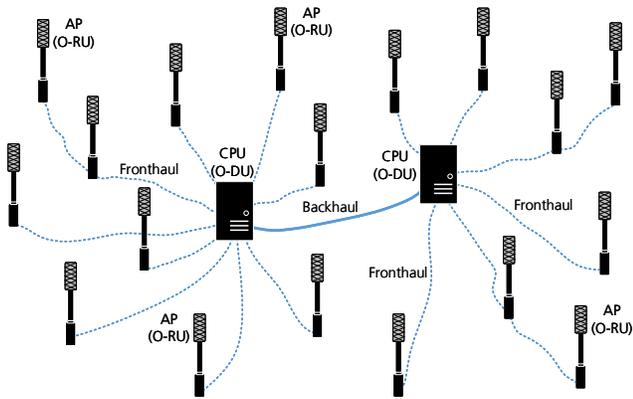
Fig. 13. Conventional cell-free mMIMO architecture with its front- and backhaul links.
