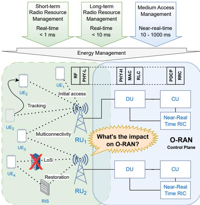
Fig. 1. RAN Management requirements (top) and the main challenges that smart factory networks (left) bring to the O-RAN control plane (right).
