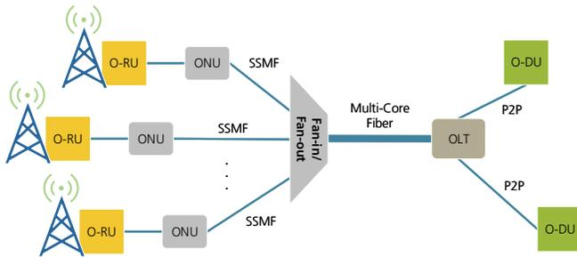
Fig. 12. Deployment example of an SDM-PON system.
