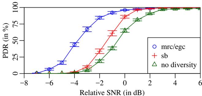
Figure 5. Experimental PDR for a two-branch diversity system [37].
