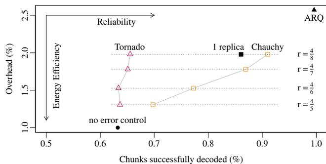
Figure 4. Reliability gain achieved by the different error control strategies and code rates  $r$  versus energy efficiency [33].
