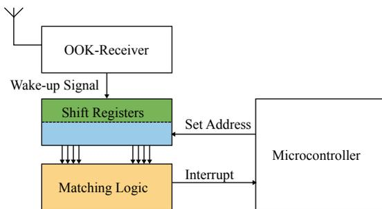
Figure 3. Basic Architecture of our SWuRx platform [28].
