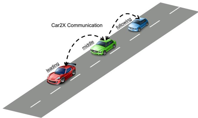
(a) Platooning as a CPS: Cars control their speed and acceleration to build a stable platoon using vehicular networking
