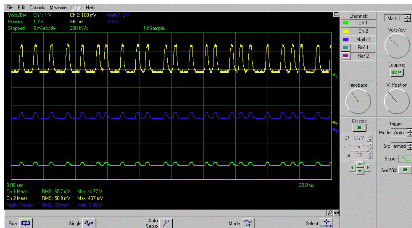
Figure 2: Reception at 11Mb/s of 64 byte packets
