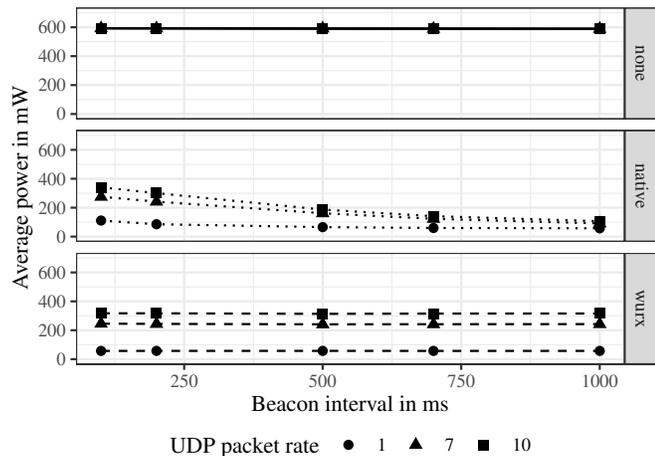
Fig. 9. Simulation results with 32 nodes. The WuRx-approach particularly saves energy for low data rates.
