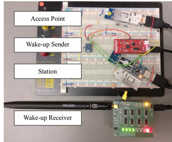
Fig. 4. Hardware prototype consisting of two WLAN dongles and a wake-up sender and receiver.
