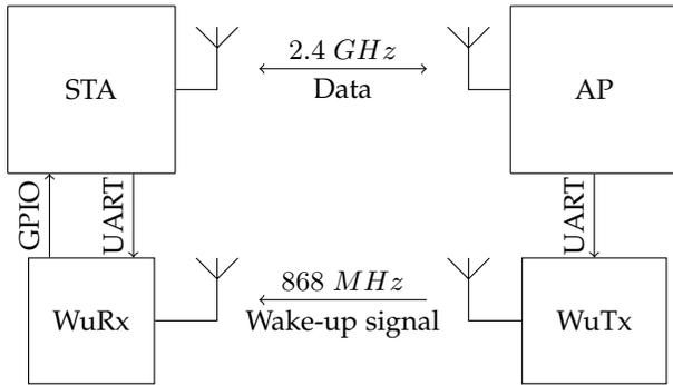
Fig. 3. Block diagram of our prototype with wake-up extension
