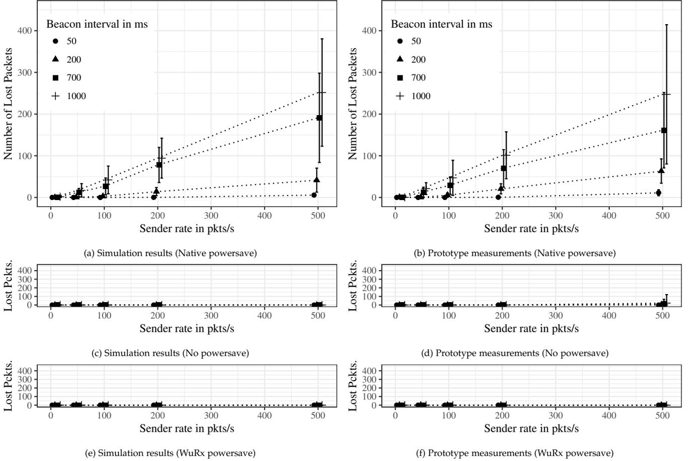
Fig. 8. Effects of bursty traffic: In native power mode packets can be lost if they arrive at a high rate and can not all be buffered.
