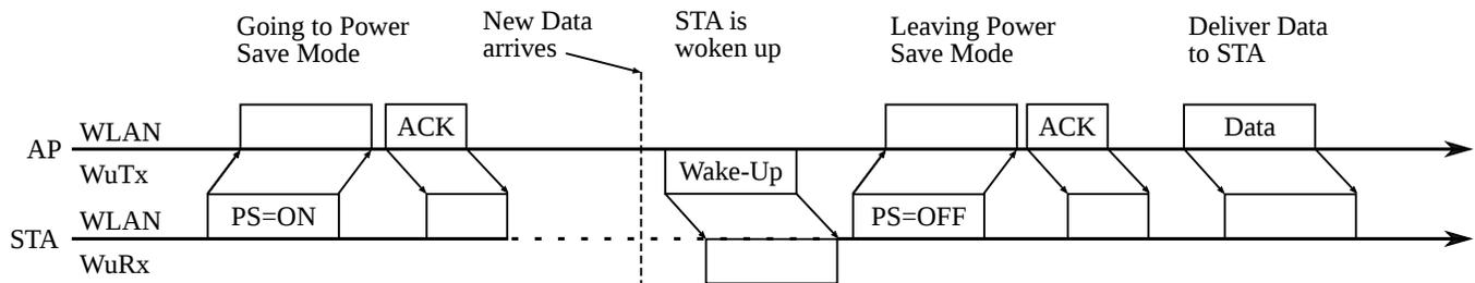
Fig. 2. Packet exchange using the WuRx system. Instead of waiting for the next Beacon, the STA is woken up immediately. The dashed line indicates that the main transceiver is in sleep mode.
