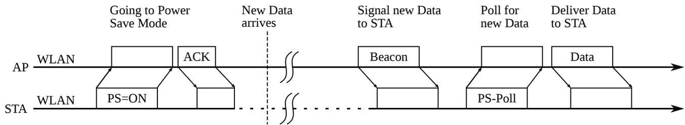
Fig. 1. Example of power save (PS) frame exchange defined in the IEEE 802.11 standard using the polling protocol. The dashed line indicates that the main transceiver is in sleep mode.
