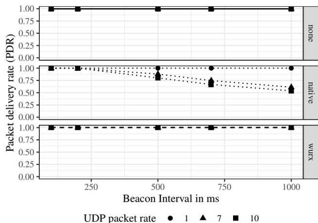
Fig. 10. Packet delivery ratio (PDR) for scenario with 32 nodes and a buffer size of 50 packets. The AP has to drop packets in native power save mode.
