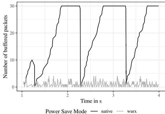
Fig. 11. Buffer fill level at the AP (maximum 30 packets). In native power save mode packets have to be dropped because the buffer runs full before the next beacon interval.
