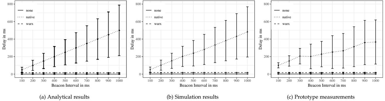
Fig. 7. Delay performance results: A higher beacon interval increases the delay in native power save mode; without power save or in WuRx mode, the delay is considerably lower. Error bars show the standard deviation.
