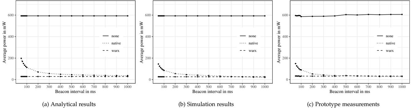
Fig. 6. Energy performance results: In native power save, the energy consumption depends on the beacon rate; the WuRx operation has a low energy consumption regardless of the beacon interval.
