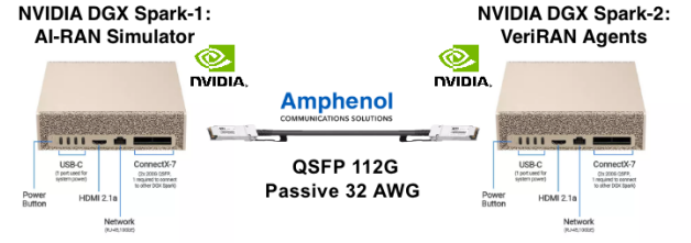
Figure 1: Two-Spark AI-RAN system architecture; connected via Amphenol Cable QSFP-to-QSFP 112G, 32AWG.
