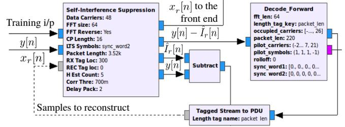
Figure 4. A screen shot of the most relevant blocks of our Full-Duplex Relay implementation in GNU Radio Companion.
