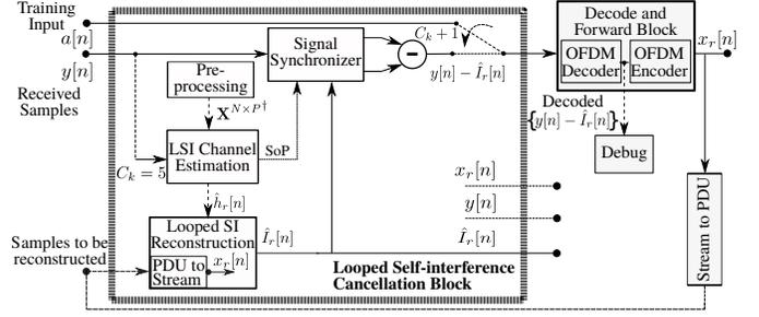
Figure 3. Detailed baseband level block diagram of our novel LSI suppression module for full-duplex relay implementation.
