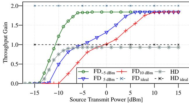
Figure 9. Achieved throughput gains with FD relaying over HDR at different transmit power levels of the relay node.
