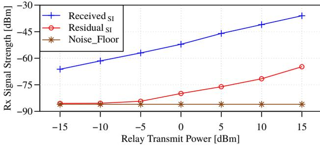
Figure 6. Looped SI suppression performance of the implemented FDR in digital domain with increasing transmit power levels of the relay node.
