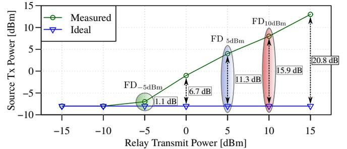
Figure 8. Required source transmit power levels to maintain PDR of 90% for a given relay transmit power. The circled points highlights the 90% PDR values of Figure 7.
