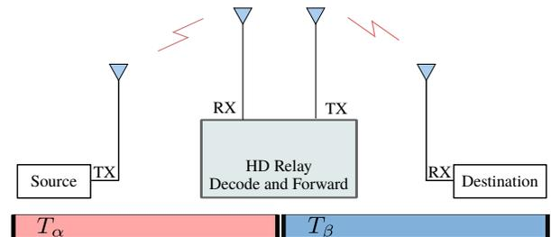
Figure 1. A typical two hop relay system operating in Half-Duplex mode.
