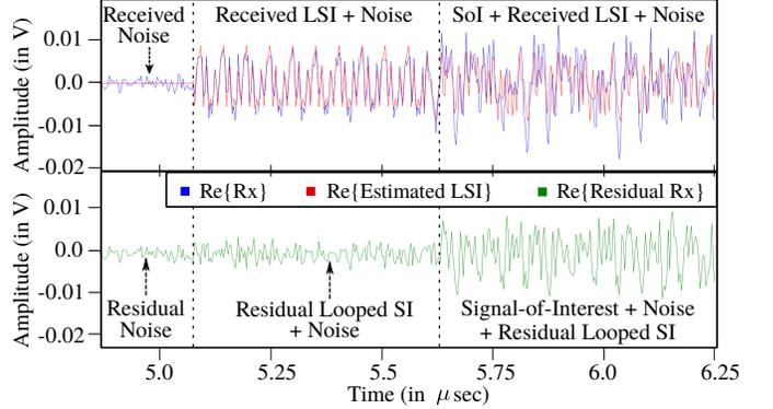
Figure 5. Snapshot of real-time LSI cancellation performance of our relay node under full-duplex mode.
