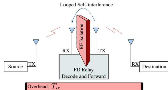
Figure 2. A two hop relay system operating in Full-Duplex mode.
