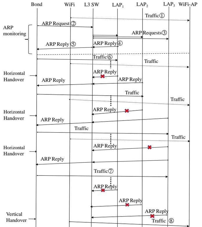
Figure 3: Packet flow diagram of Li-Wi
