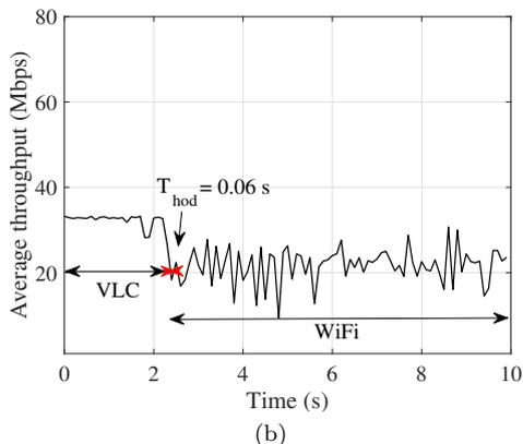
Figure 12: Li-Wi performance applied on a hybrid architecture experiencing only vertical handover using (a) Default (b) Redundant schedulers.
