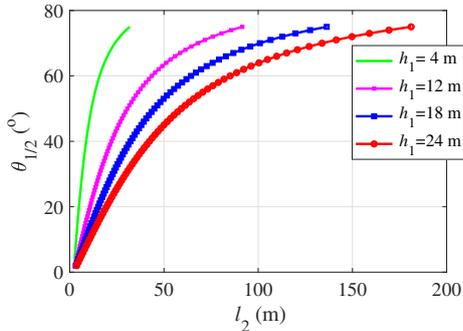
Figure 9: LAP's FOV as a function of half power angle for a range of vertical link spans.
