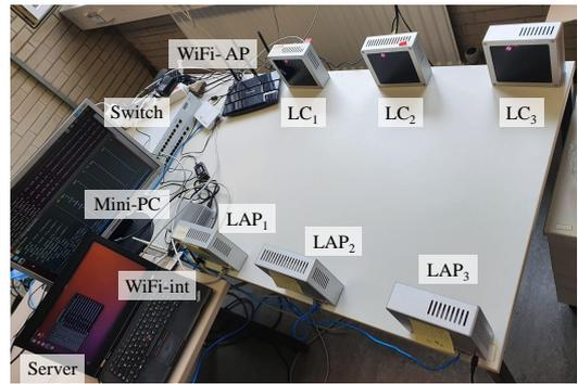
Figure 4: Experimental indoor Li-Wi setup
