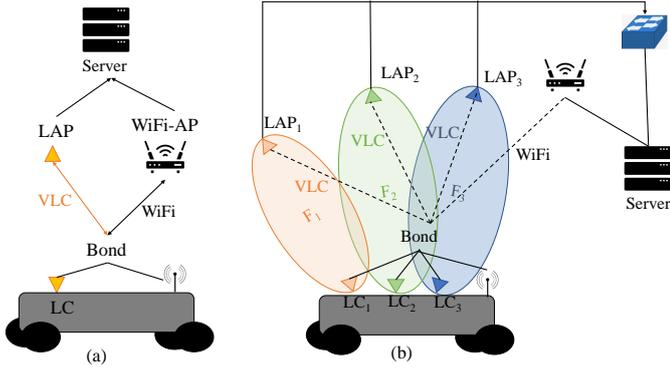
Figure 5: Link aggregation between VLC and WiFi use case scenarios
