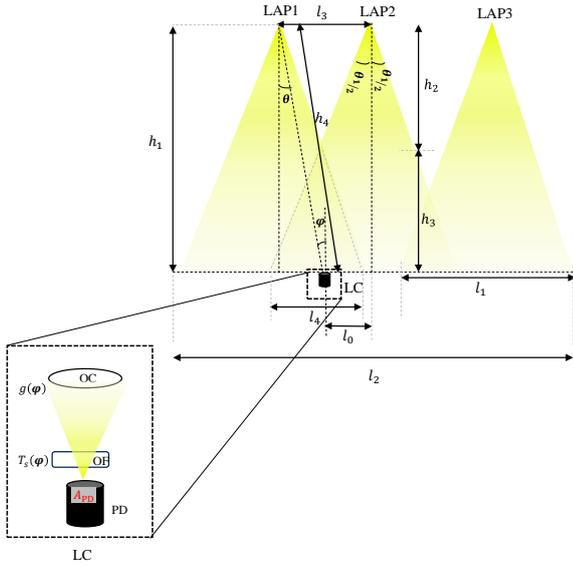
Figure 10: Configuration of an indoor V-VLC system.
