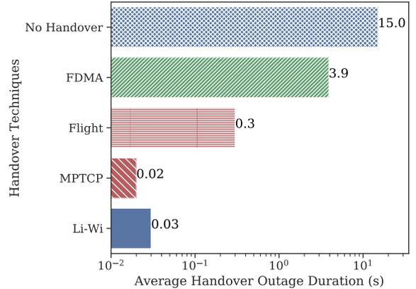
Figure 1: Comparison of horizontal handover outage duration for different handover methods.
