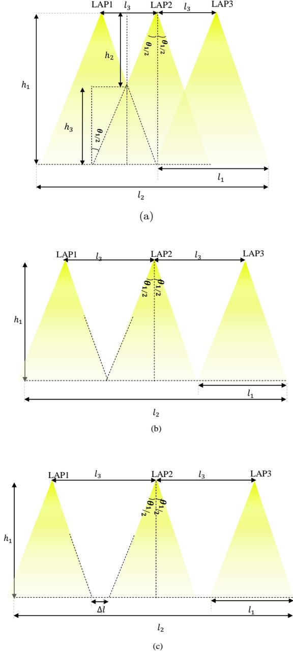
Figure 8: Illumination profiles with: (a) overlapping, (b) non-overlapping with no illumination gaps, and (c) non-overlapping with illumination gaps scenarios.
