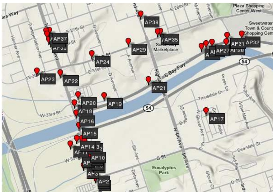
Figure 7.7: A Residential Area in San Diego - Some APs configured on channel 6
