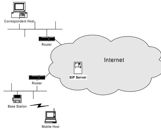
Figure 4.10: Network architecture in the *Extended SIP mobility* approach
