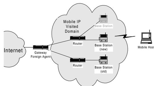
Figure 4.2: Network architecture for Mobile IP with hierarchical foreign agents
