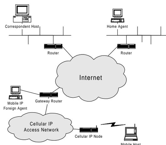
Figure 4.6: Cellular IP network architecture
