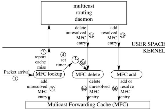
Figure 4.2: Interaction between kernel, multicast routing and paging daemon
