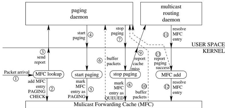
Figure 4.3: Interaction between kernel, multicast routing and paging daemon
